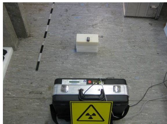
Figure 11: Measuring configuration for a distance of 50 cm.
