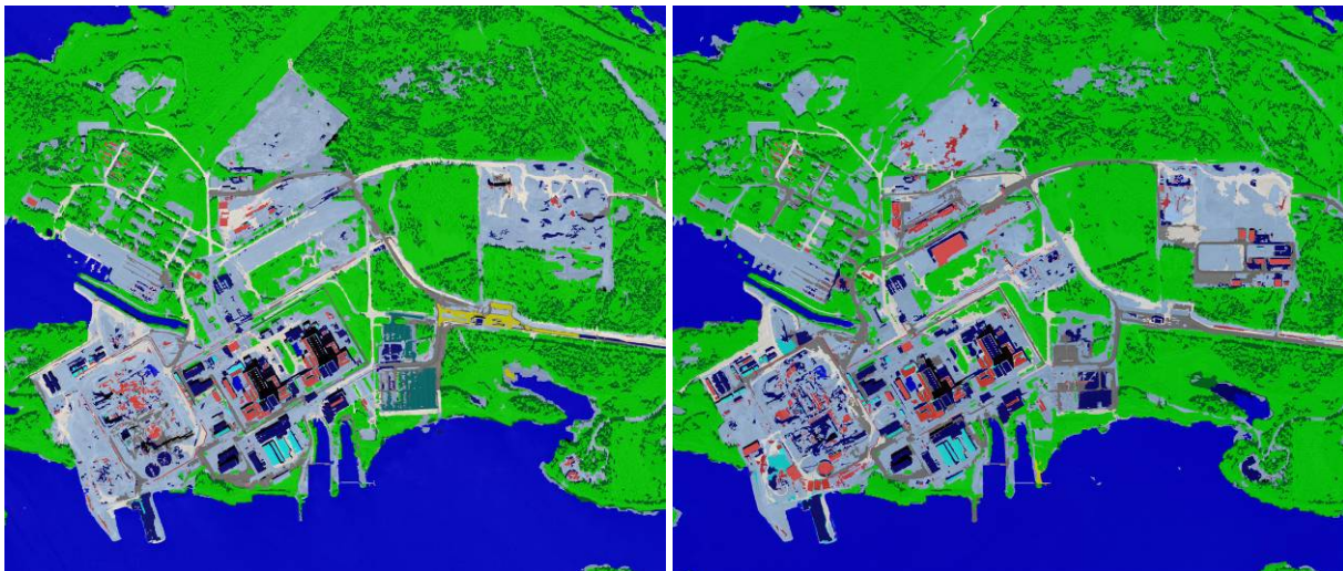
Figure 7: Result of applying the object-based image classification to the 2005 (left) and 2006 (right) Olkiluoto images. A semi-automated change analysis can be achieved by fusing the change detection and image classification components.
