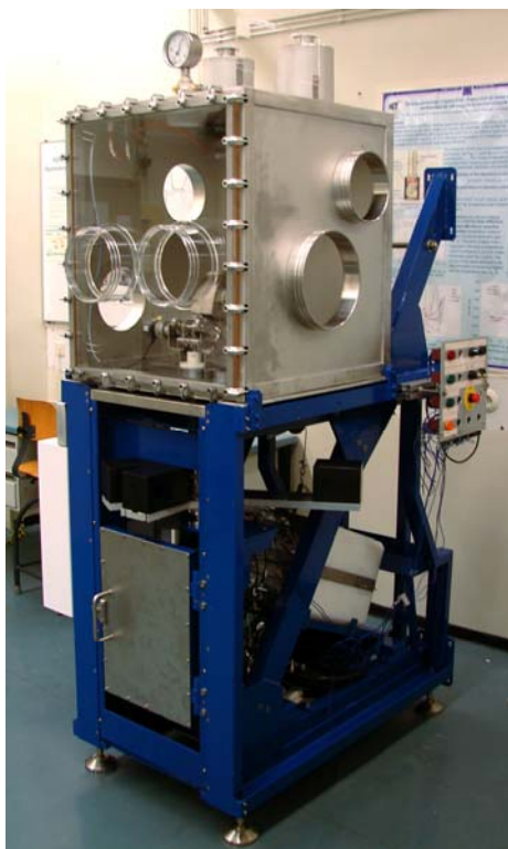
Fig. 8. Photograph of the compact NDA station (Ge detectors removed) prior to the installation at the hot cell.
