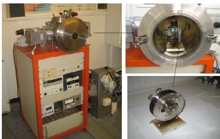
Figure 1: Carburization device (left) and a vacuum chamber with a filament magazine (right).
