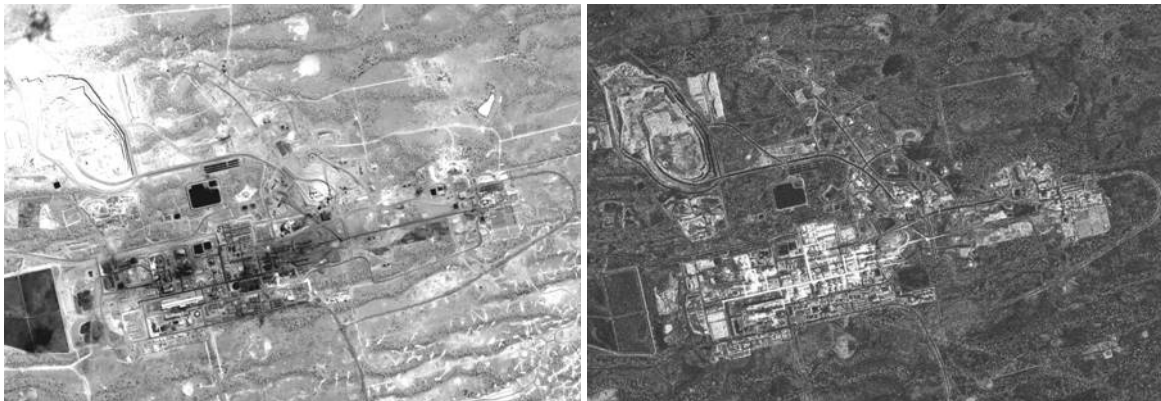
Figure 1: WorldView 0.5 metre optical image acquired on Aug. 18, 2008 (left) and TerraSAR-X 1 metre image acquired on Feb. 14, 2009 (right) showing the Olympic Dam mine in Australia.
