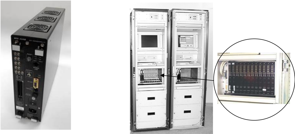
Figure 1: For small systems the Web Adam (left) is ideal but for large systems, the VXI system (right) can support 96 detectors
