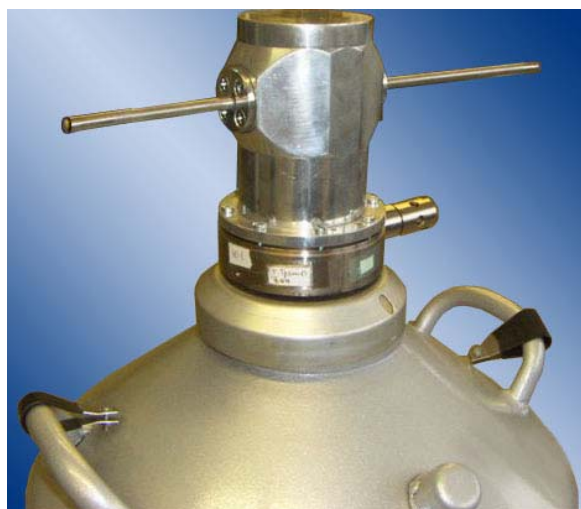
Fig. 1. Flow-type HPGe detector with through channel
