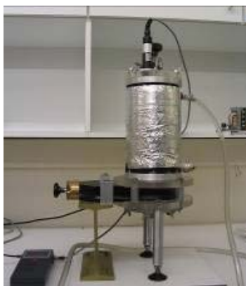
Fig. 1: Set-up of the aerosol deposition chamber
