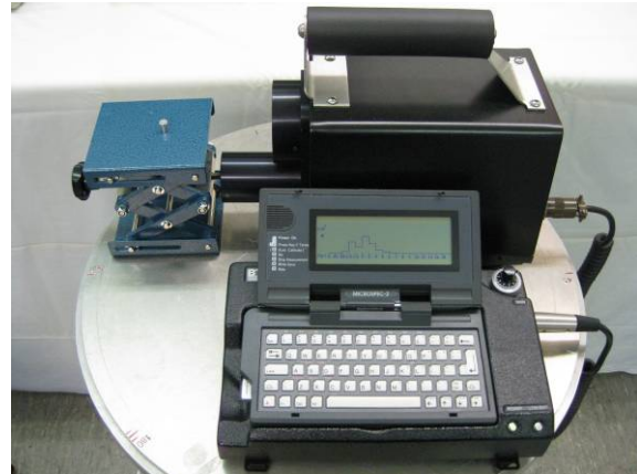
Figure 2: N-probe neutron spectrometer. The hand-held computer placed in the front is displaying the measured energy spectrum. A neutron source is placed on the little lifting plate. The N-probe is behind the computer with the two detectors on the left side, liquid scintillator at the top and ^3\text{He} tube below.
