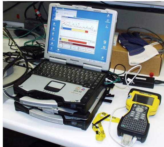
Figure 5: Pocket computer control unit (“Ranger”) and remote display on laptop screen, data transfer via serial cable.
