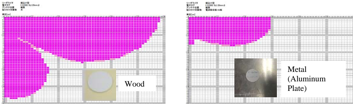
Figure 2. Directional characteristics on wood and metal (I-CODE SLI Circle \phi 20\text{mm} ).
