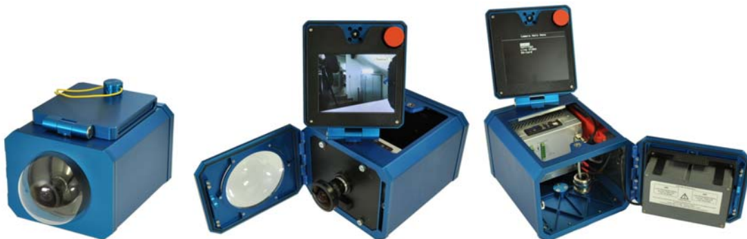
Picture 2: NGSS Data Generator Prototype
