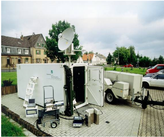
Figure 1: Transportable container, gamma and neutron measuring devices in front. On the right side power generator on separate trailer.
