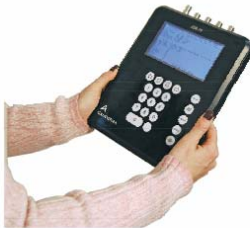
Figure 1: JSR-15 Hand Held Multiplicity Shift Register. There is a single shifter register input and two extra scalars. The JSR-15 weight is 1.7 kg and its dimensions are 254x203x32 mm
