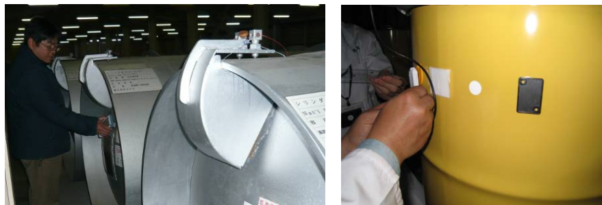
Figure 7. Reading I-CODE SLI tag using PDA-type reader/writer on 48Y cylinder (right). Several RFID tags on 200 liter drum (left).
