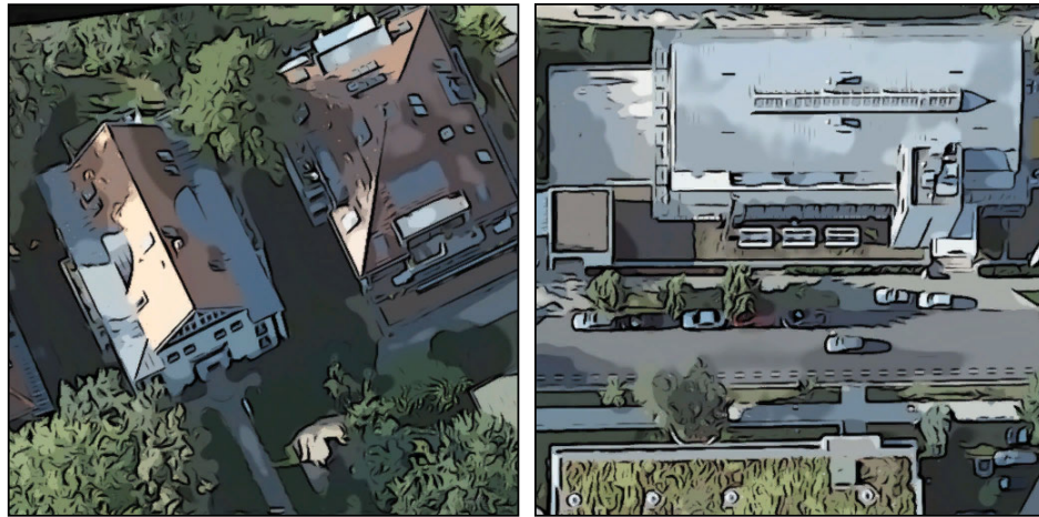
Figure VII.1: Abstracted aerial images created using the proposed method for tile-based image filtering. Here, the flow-based bilateral filter of Kyprianidis & Döllner (2008) was used for processing.
