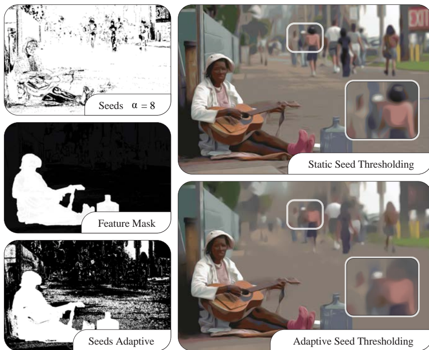
Figure VII.18: Using adaptive thresholds for the placement of color seeds to control the level of abstraction for image features. (top) Static thresholds \alpha = 8 , (bottom) adaptive thresholds \alpha \in [3, 11] selected according to an importance mask to increase the LoA for features in the background.
