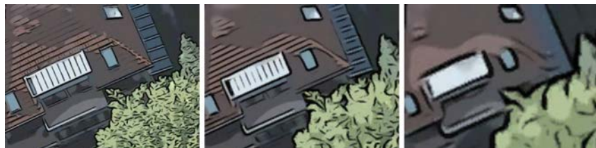
Figure VII.5: Level of abstraction by means of trilinear filtering. The viewpoint distance decreases linearly from left to right. The greater the viewpoint distance, the fewer details are depicted at the roof of the building and the tree.
