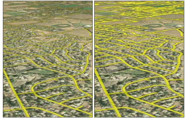
Figure III.23. View-dependent design of transportation networks using (left) no scaling, and (right) a distance-based scaling function. Image courtesy by Vaaraniemi et al. (2011).
