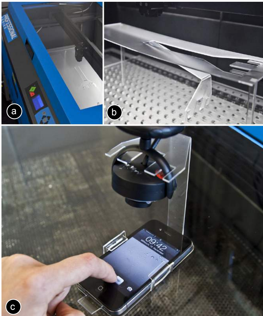
Figure 74: LaserOrigami fabricates 3D structure by bending rather than using joints, thereby eliminating the need for manual assembly.
