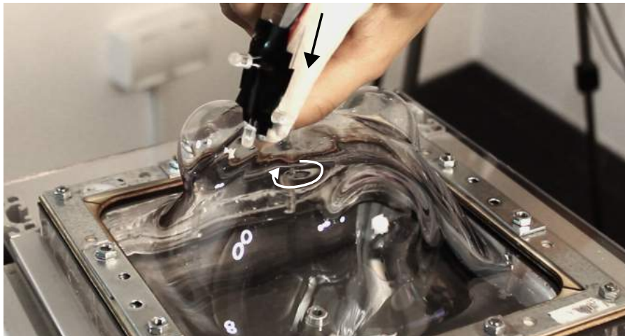
Figure 101: Extruding the eyes inward with vacuum.
