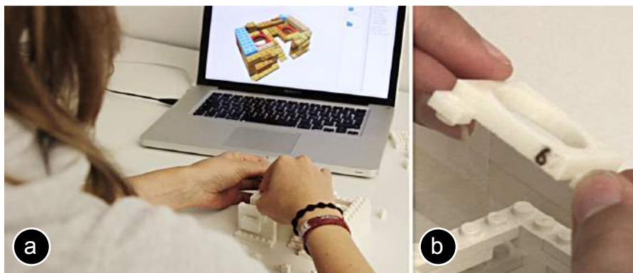
Figure 14: (a) Assembly instructions highlight the next brick in blue. (b) Each 3D printed part has a unique ID.
