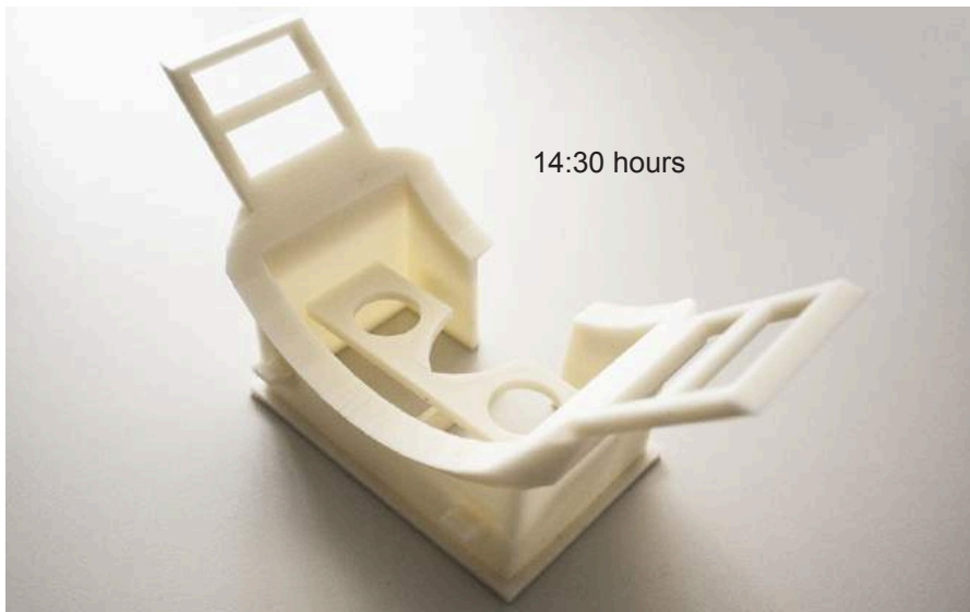
Figure 8: Fabricating this head-mounted display body requires overnight printing, slowing down the feedback cycle to only one iteration per day.
