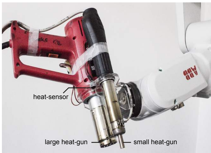
Figure 103: The larger heat gun allows heating coarse base shapes. We use the small heat gut for finer details. The temperature sensor notifies FormFab when the material reaches its compliance point.
