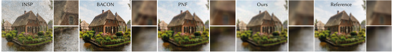
Fig. 12. A qualitative comparison between INSP [Xu et al. 2022], BACON [Lindell et al. 2022], PNF [Yang et al. 2022], and our approach using a Gaussian kernel. INSP approach does hardly perform any filtering, when the kernel is larger, such as our approach supports, but suffers from noise. BACON fairs better, but shows ringing at high-contrast edges such as the house against the sky, while PNF also struggles to produce low-pass filtering results.
