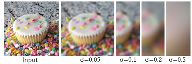
Fig. 10. Gaussian 2D image blur of the input signal, with increasing bandwidth. It can be seen how our approach works also for large kernels.
