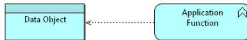
Figure 6.1: Data object and application function concepts from the application layer of ArchiMate, Adapted from: ArchiMate ® 2.0 specifications ( The Open Group (2012) )
