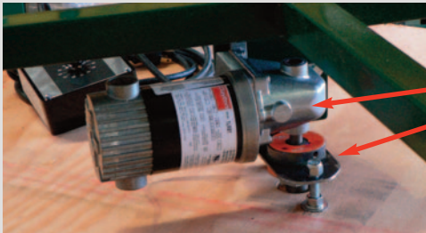
Inverted view of turn table drive
