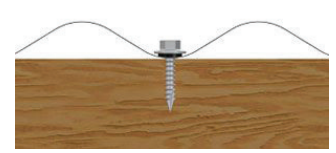
Valley fixed into timber
