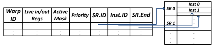
Figure 5: Fetch Logic: Assist Warp Table (contained in the AWC) and the Assist Warp Store (AWS). Figure reproduced from [115].
