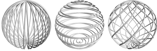
Figure 2: Basic motions of a Clelia curve. From left to right are meridional ( \{1\}\{20\} ), parallel ( \{20\}\{1\} ), and mixed ( \{10\}\{11\} ) motions.
