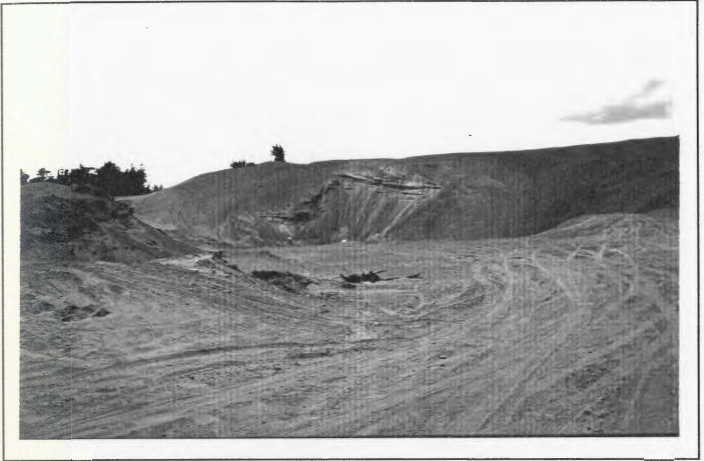
Plate 6.2 - The exposed and eroded face at Section A15 showing horizontal bedding and trough cross-bedding. The section is 21 m high, 100 m wide and faces towards the east. Beds within the exposure dip at an angle of 15^{\circ} towards the northeast.
