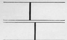
As image will appear when Range Finder is set for a distance beyond the correct one.
