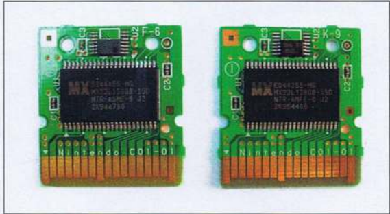
△ Here's what they can fit inside a DS cart – nothing more than a ROM chip and some rewritable memory. The add-ons such as motion sensors or rumble motors that we're used to seeing on Game Boy will go in the separate GBA cart slot. In fact there's a space in every DS game box for holding a GBA cart, so some games are likely to come packaged as a two-cart set.
