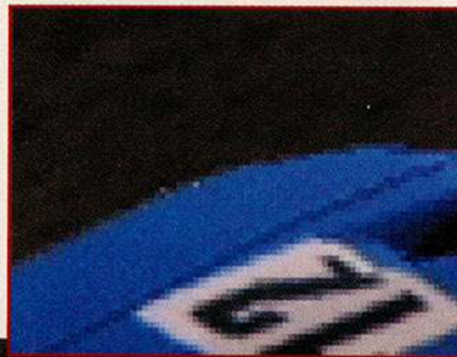
See how the edges of this R: Racing Evolution car are feathered with light blue and gray pixels to smooth out the transition? That's anti-aliasing.
