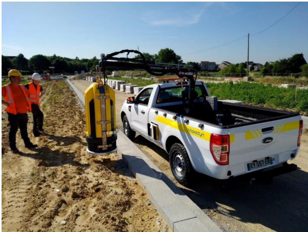
Max extension of the Dynaplaque Maxidyn.
