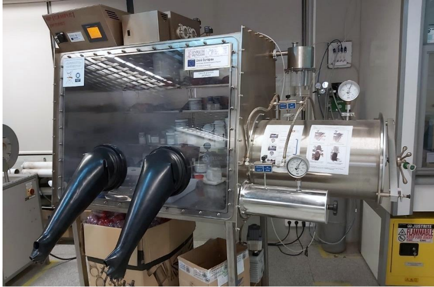
Fig. 9. Glove box of the Jacomex manufacturer, model GP Campus.
