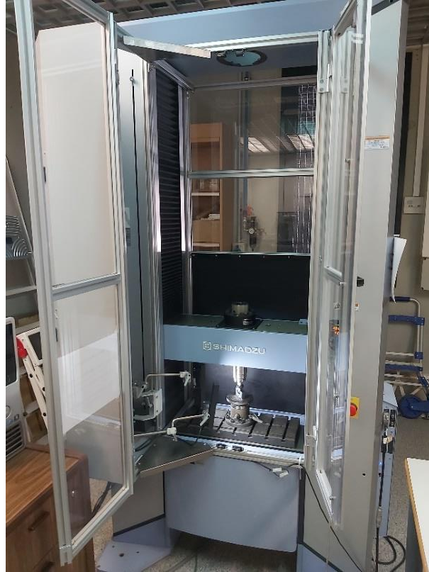
Fig. 35. Shimadzu Autograph AG-100 KN Xplus universal testing machine.
