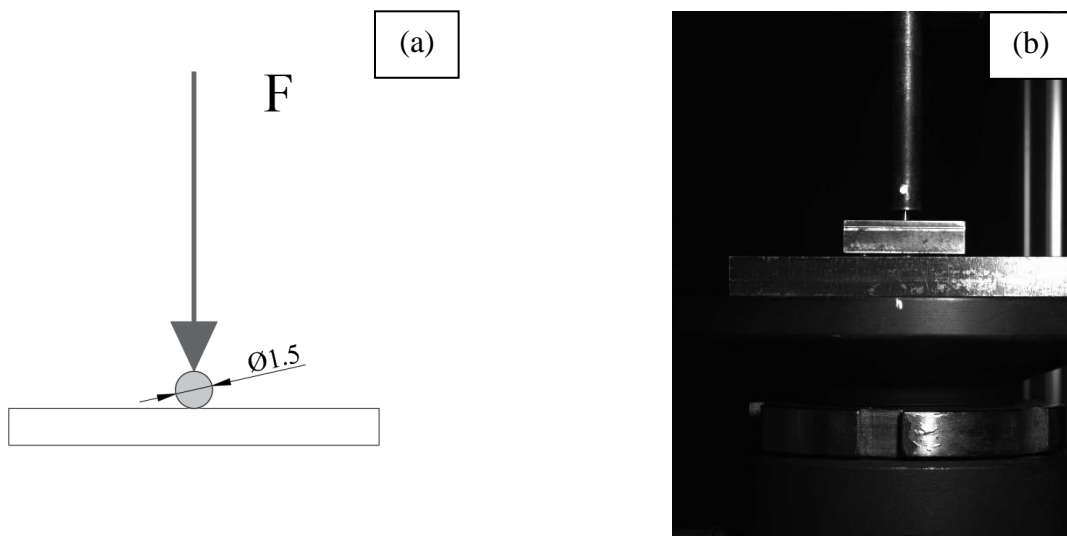
Fig. 42. (a) Dimensions of the ball used during small punch test in mm and (b) small punch test procedure.
