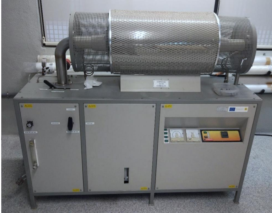
Fig. 13. High vacuum furnace of the manufacturer Carbolite Gero Limited, model HVT 15-75-450.
