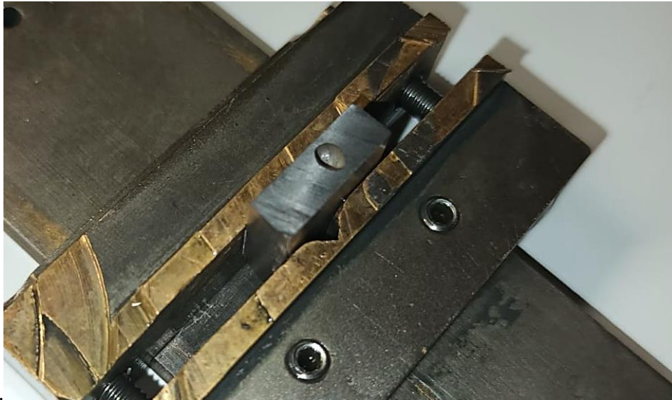
Fig. 60. Macropore in the TNZT casting sample.
