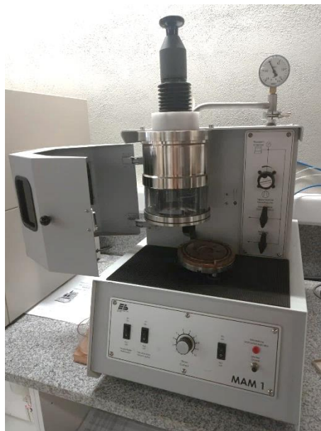
Fig. 16. Arc melting furnace of the Edmund Bühler GmbH manufacturer, model MAM-1.
