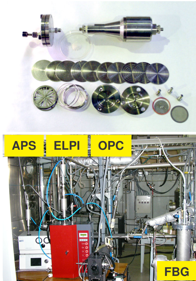
Fig. 50. Instrumentation used for aerosol characterization and generation.
