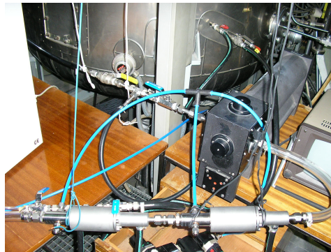
Fig. 58. OPC-ELPI configuration with diluters for a DEHS test.
