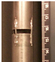
Fig. 17. Guillotine break used in the CAHT experiments.
