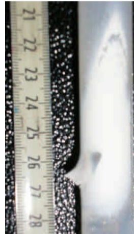
Fig. 62. Tube deposits detail for a \text{TiO}_2 experiment.
