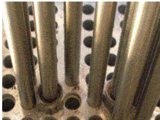
Fig. 54. Tubes selected for aerosol deposits collection and U-rings picture.
