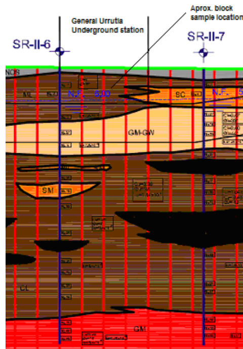
Figure 6.3 Soil profile at the General Urrutia underground station where the block sample of the VSS was retrieved
