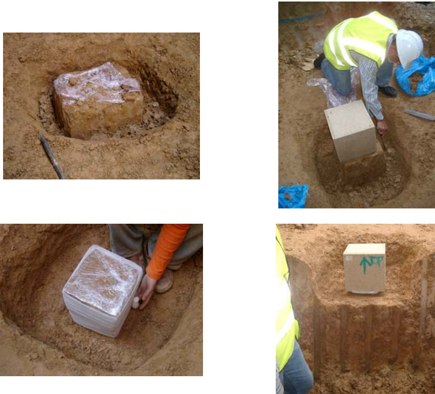
Figure 6.4 Sampling process of the intact block of the VSS obtained from the excavation works of the T2 underground line extension to the south of the city of Valencia at the General Urrutia underground station
