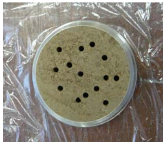
Figure 3.9 Oedometer sample after holes were drilled
