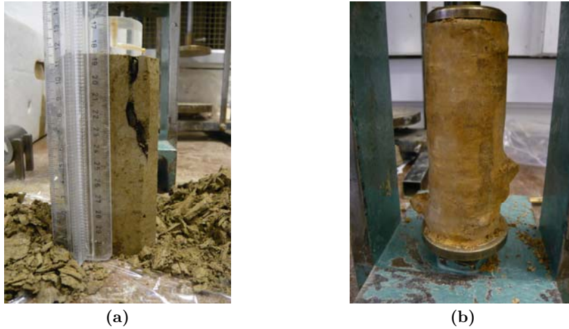
Figure 3.12 Trimming procedure of the (a) BRS and (b) VSS intact samples
