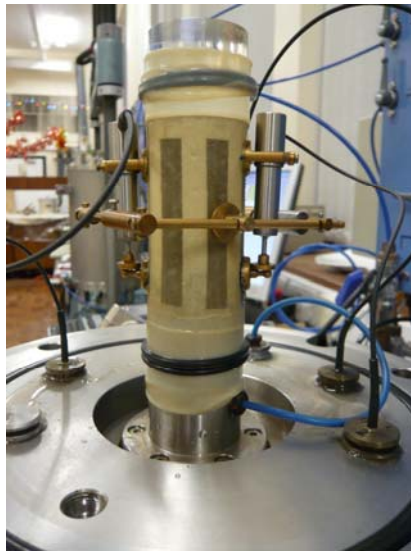
Figure 3.5 Local LVDTs for measuring axial and radial strains of samples
