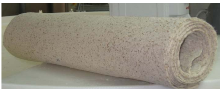
Figure 4. Nonwoven sheet rich in natural fiber rolled up, obtained by wet laid technology.
