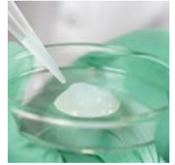
Image: Hydrogels swell and shrink in response to environmental signals. CC BY-SA 4.0.
