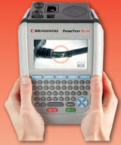
The ProTag Elite System tests portable appliances & RCDs, takes asset photos, prints Elite UV resistant test tags & downloads results to PC. Mains & battery powered. Faster testing & asset management for mining, construction, factories & workshops.
