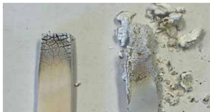
Side-by-side comparison: The team's proposed power pole insulation material (left) next to silicone following a fire-resistance experiment.
