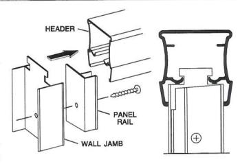
Cut the inline panel vinyls [H] to the length of the long edges of the inline glass panel [J] and press them onto the edges of the panel. Stand the panel upright on the tub track [A] and press it into the mounted inline panel rail [G]. Press the second panel rail over the other edge of the glass panel and vinyl with the bottom of the panel rail flush against the tub track.
