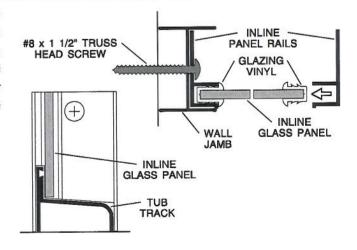
Install the third wall jamb [B] by engaging the upper end into the header [F] and sliding the jamb up against the second inline rail [G]. Plumb the center wall jamb and secure it with a #6 x 3/8" truss head screw [K] thru the exterior face of the tub track [A] and another thru the interior face of the header.
