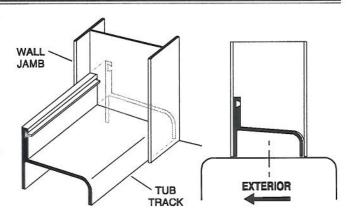
Use a level to plumb both wall jambs [B], then mark the pre-drilled hole locations on the wall. Lightly mark along both sides of the tub track [A] with a pencil, then remove all parts.
