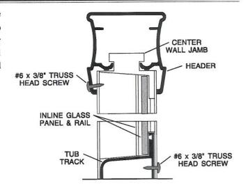
Attach the second inline rail [G] to the center wall jamb [B] with two #8-32 x 1/4" truss head screws [L] thru the top and bottom holes into acorn cap nuts [M] on the inline panel side. Slide a nylon spacer [E] onto a #8-32 x 3/8" truss head screw [N], insert into the center hole and attach an acorn cap nut.
