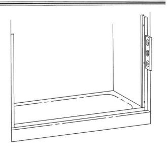
Before replacing the tub track [A], force a slight downward bow in the extrusion. This will ensure the track fits tight to the tub. Run two beads of caulk inside the penciled marks on the tub rim. Place the tub track in the exact position marked in Step #2 and seat it firmly in the caulking.
