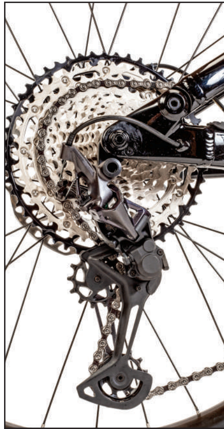
The drivetrain includes a Shimano SLX M7100 12-speed cassette with 10-51T offers plenty of range.
