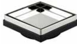
Tile Drains Stainless Steel Grade 316 Capacity - 35 l/m 130 x 130 mm Vertical Outlet Dia. 74 mm
