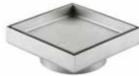
Heavy Duty Tile Drain Stainless Steel Grade 316 2.0 mm Thick Vertical Outlet 102 mm Outlet Capacity - 35 l/m 146 x 146 mm
