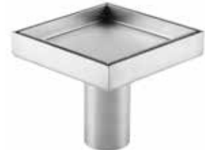
Heavy Duty Tile Drain Stainless Steel Grade 316 2.0 mm Thick Vertical Outlet 50 mm Outlet Capacity - 35 l/m 146 x 146 mm
