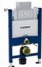
Duofix Concealed Cistern for Wall Hung WC with Alpha Concealed Cistern 120 mm for Dry Wall Construction or Prewall Installations or Room-Height Installation with Fastening Material Thickness 170 mm Height 820 mm
