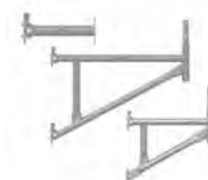
RINGLOCK ROAD BRACKET SWS-U-RLBB12 12" - ONE BOARD WT. 4 LBS SWS-U-RLBB20 24" - TWO BOARD WT. 21 LBS SWS-U-RLBB30 36" - THREE BOARD WT. 24.5 LBS
