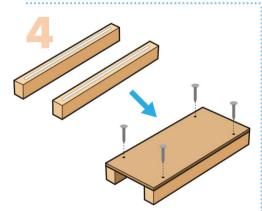
**Step 4** — Stand both **drawer side pieces** up on their narrow edges. Glue the **drawer bottom piece** on top. Ensure all corners are even. Nail them together with 4 **nails**.
