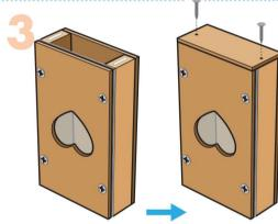
**Step 3** — Stand the **project** up with the heart window upside down. Glue the **bottom piece** on top, ensuring all edges are even. Nail them together with 2 **nails** to form a **box**. Set the **box** aside for now.
