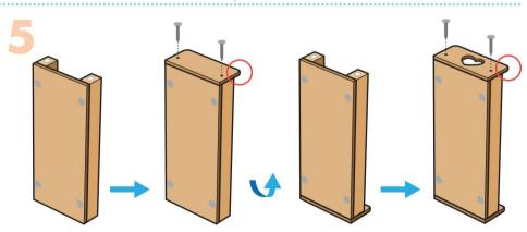
**Step 5** — Stand the **project** up. Apply glue to the top edge of the **drawer side pieces**. Place the **drawer back piece** on top, aligning the square corners with the bottom edge. The rounded corners will overhang. Ensure the side and bottom edges are even. Nail them together with 2 **nails**. Turn the **project** over. Repeat on other side with the **drawer front piece**, forming the **drawer**.
