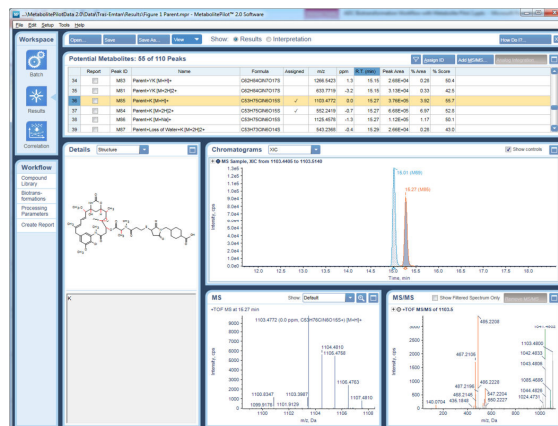
Figure 3. The results workspace of MetabolitePilot 2.0 software displaying results from the incubation of T-E with human liver lysosomes. The released payload species (payload+linker+lysine) was found at retention times 15.01 and 15.27 minutes as a pair of diastereomer peaks. The structure of the payload and linker species is displayed on the left with the amino acid of conjugation below. Also displayed is the MS and MS/MS spectra of the released payload species.
