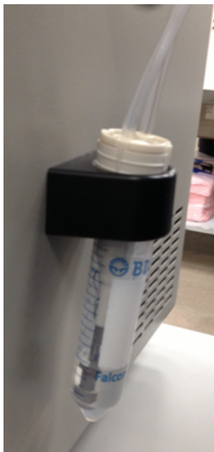
Figure 7-13 Sprayer Immersed in Liquid
