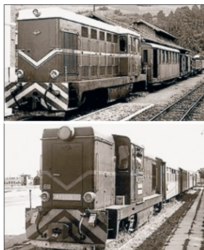
Plate 6 23 August diesel-hydraulic locomotives on the narrow gauge: at Câmpeni on the Turda-Abrud line with a mixed train including a passenger coach of 1950s vintage built by Unio of Satu Mare (above); and another at Sibiu with a rake of more modern coaches built by MEVA (Drobeta-Turnu Severin) in the 1980s for the Agnita branch
