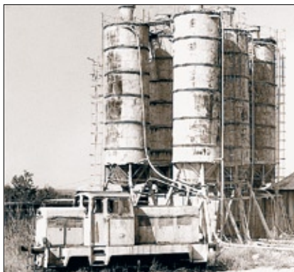
Plate 7 One of the many short industrial branches: giving access to a cement depot at Oraviţa with another diesel mechanical shunting locomotive type in the foreground: a modernised version of Class 20,000 built by 23 August in the mid-1960s
