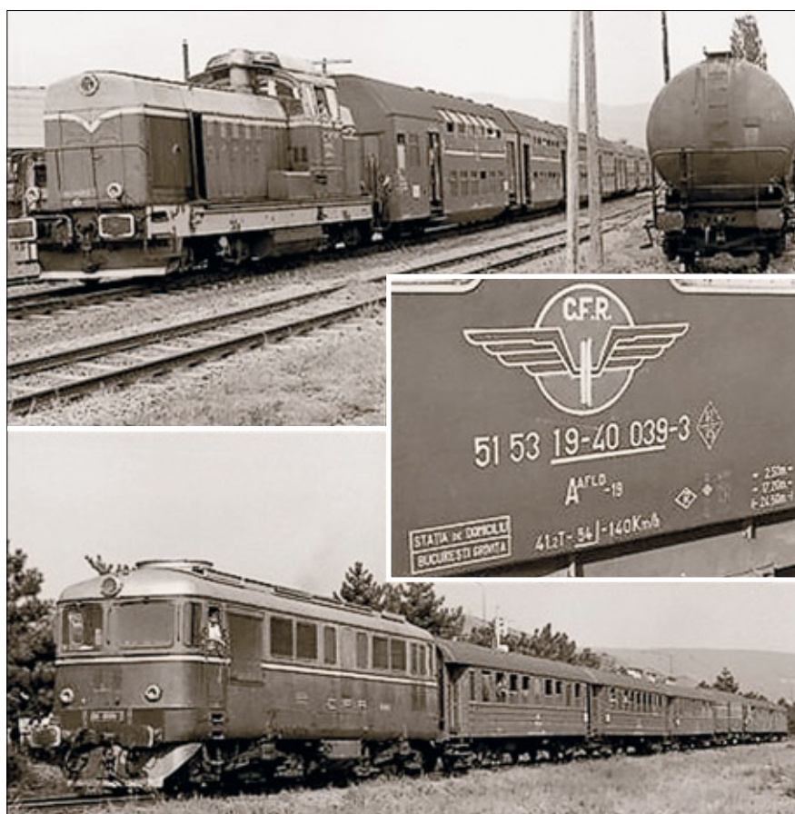
Plate 5 A 1,250hp diesel-hydraulic locomotive at Pătărlagele on the Buzău-Nehoiăşu branch with one of 120 rakes of double-deck coaches imported from Waggonbau Görlitz during 1965-73 for busy commuter lines (above); a 2,100hp diesel-electric takes a rake of coaches out of Râmnicu Vâlcea: the first three are early post-war Arad-built coaches - named 'Dimitrov Cars' because the Astra factory was renamed for a time in honour of the Bulgarian communist leader Georgi Dimitrov - formerly for express trains (but later displaced to stopping trains); with the last two new coaches built in Arad from 1964 based on a design from Pafawag Wrocław for use on stopping trains (below); and markings on a 'Type Y' coach built in the 1960s for express passenger workings
