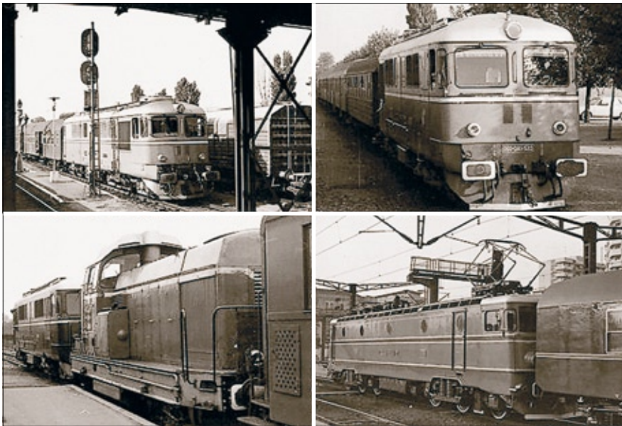
Plate 3 Diesel and electric locomotives: the 2,100hp Sulzer diesel-electric at Slatina (top left) and Alexandria (top right). Another 2,100hp diesel-electric pilots a 1,250hp diesel-hydraulic on a Craiova-Calafat stopping train (bottom left); and a 7,100hp electric locomotive enters Bucharest's Gara de Nord (bottom right)
