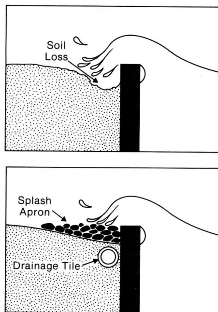
Figure 2. Storm waves frequently overtop erosion control structures. When they do, the land behind the structure should be protected with a splash apron. Drainage tile behind the structure can remove excess water.
