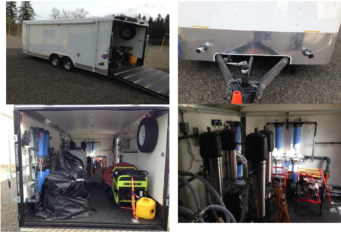
Figure 6-18. Selected Photos from Clackamas River Water’s Emergency Water Treatment Trailer
