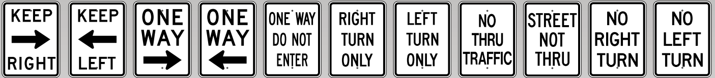
18" x 24" R4-7A(R)9 18" x 24" R4-8A(R)9 18" x 24" R6-2R(R)9 18" x 24" R6-2L(R)9 18" x 24" R-63(R)9 18" x 24" R5-805(R)9 18" x 24" R5-804(R)9 18" x 24" R-95(R)9 18" x 24" R-94(R)9 18" x 24" R3-1A(R)9 18" x 24" R3-2A(R)9
