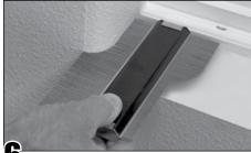
Use a contour gauge to copy the radius of the bull nose.
