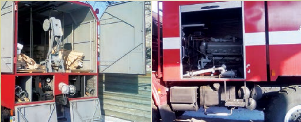
Figure 3.3. Mobile pumping (fire machines) to supply water to the steam generators in emergency modes in case of loss of power supply for own needs
