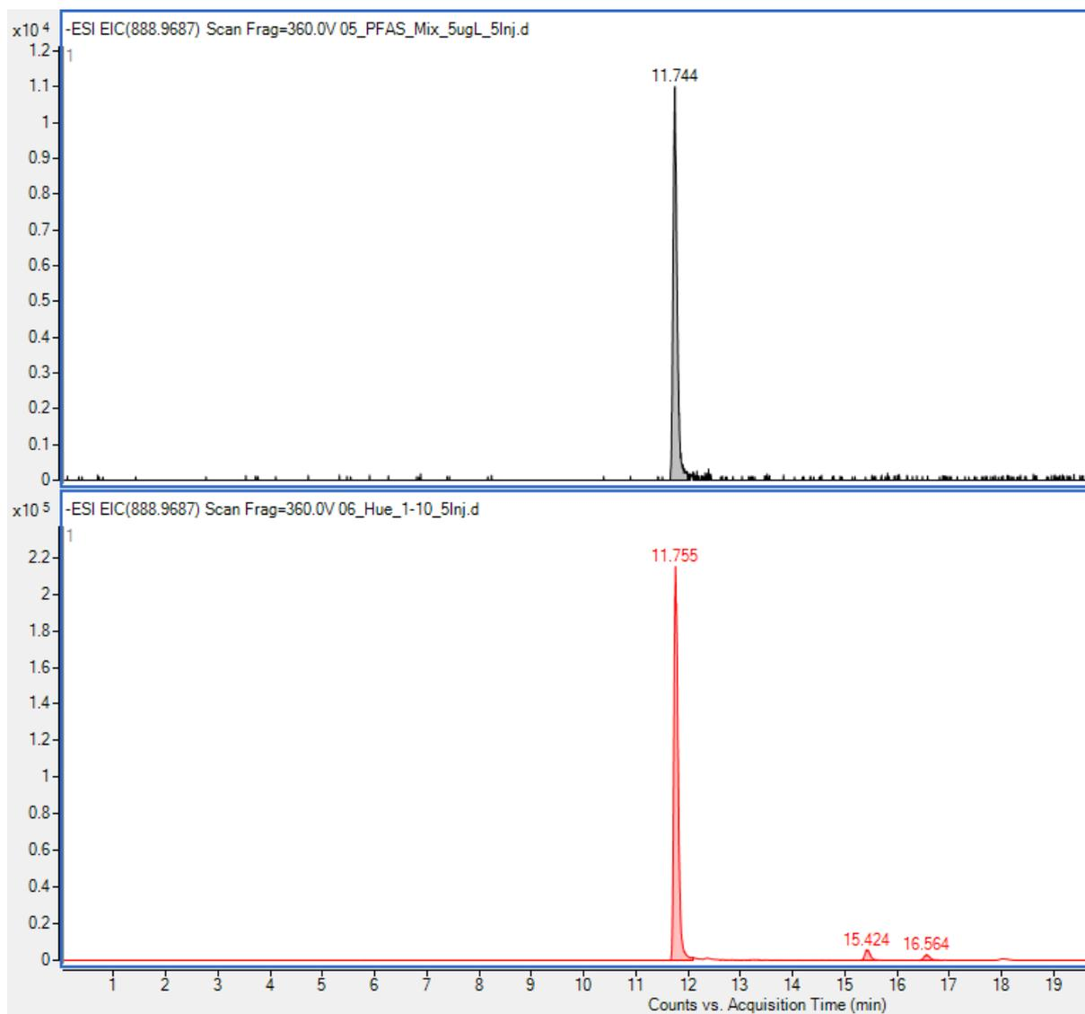
**Fig. S1.7** Top: EIC of 6:2 / 8:2 diPAP standard 5  $\mu\text{g/L}$ , bottom: 1/10 dilution of sample 1. TriPAP peaks are visible in sample 1
