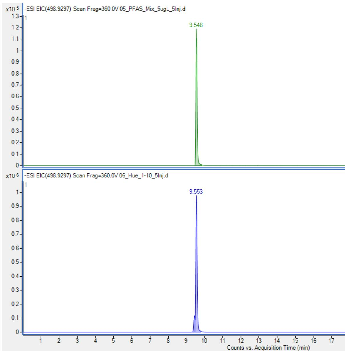
**Fig. S1.4** Top: EIC of PFOS standard 5 µg/L, bottom: 1/10 dilution of sample 1
