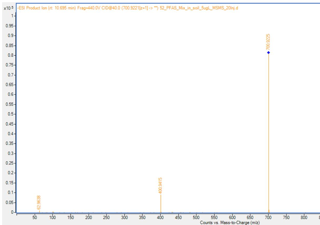
**Fig. S1.9** Recorded MS/MS spectrum of C6 PFPIA standard 5 µg/L @ 40eV
