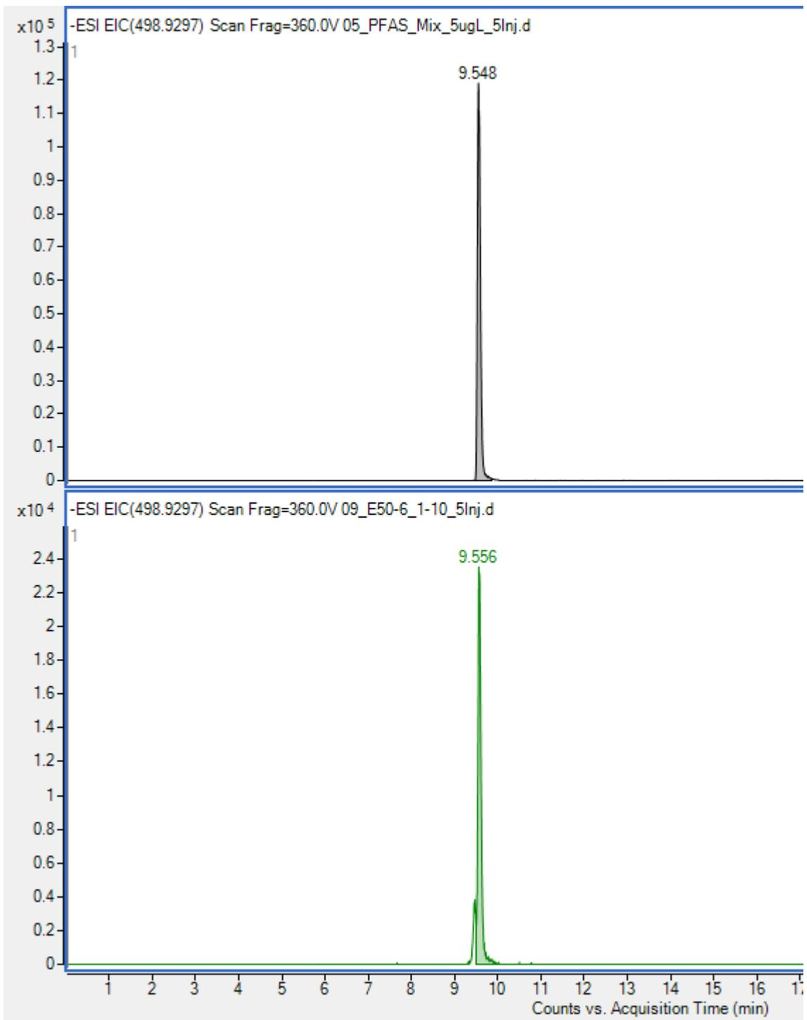
Fig. S1.33 Top: EIC of PFOS standard 5  $\mu\text{g/L}$ , bottom: 1/10 dilution of sample 4
