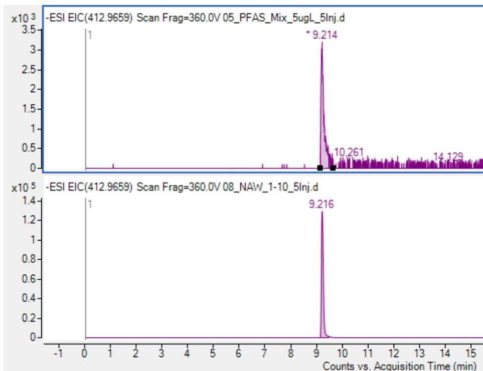
Fig. S1.46 Top: EIC of PFOA standard 5 $\mu$ g/L, bottom: 1/10 dilution of sample 2
