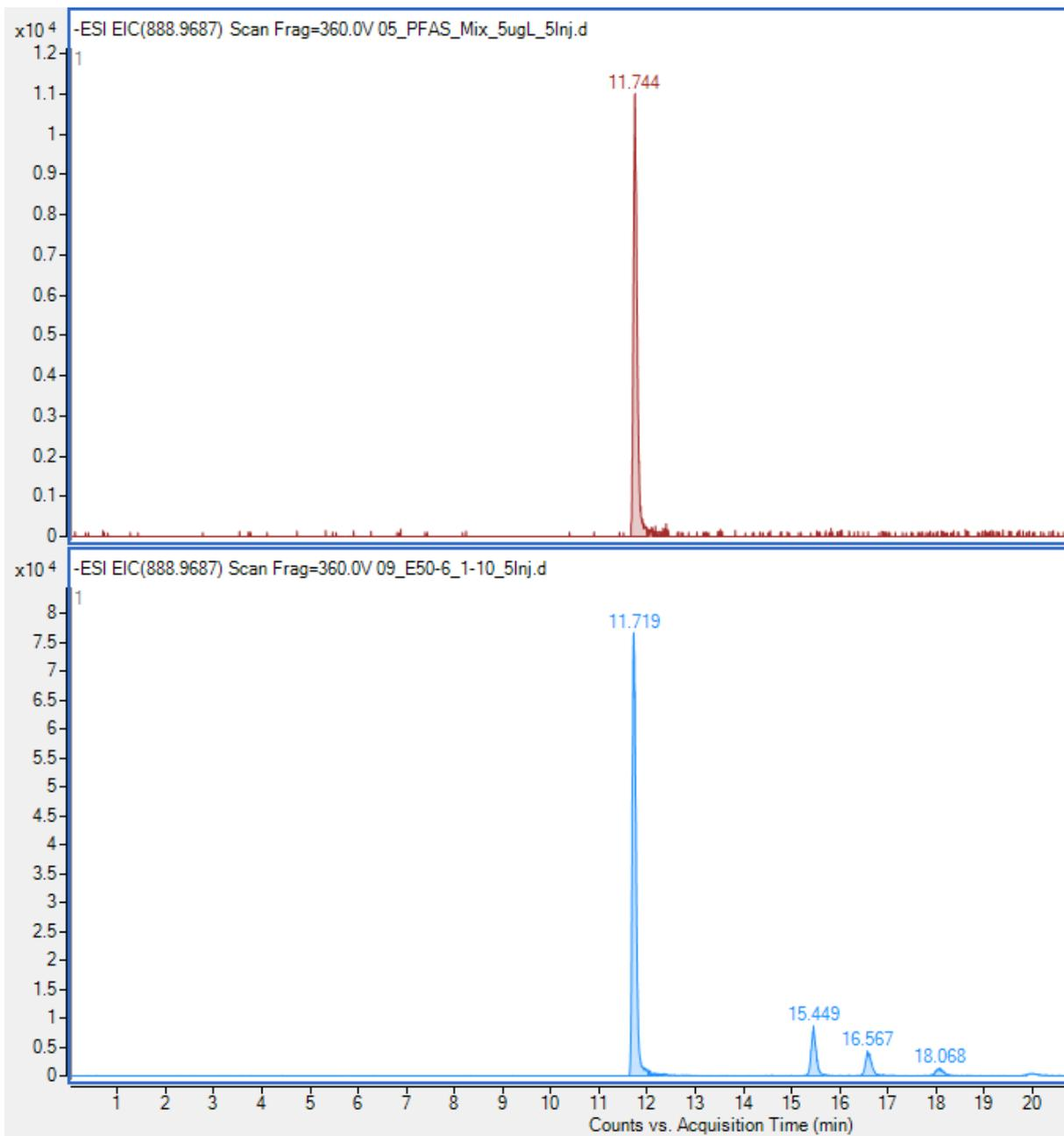
**Fig. S1.36** Top: EIC of 6:2 / 8:2 diPAP standard 5  $\mu\text{g/L}$ , bottom: 1/10 dilution of sample 4
