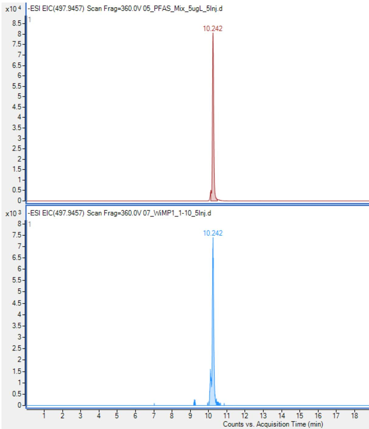
Fig. S1.25 Top: EIC of FOSA standard 5  $\mu\text{g/L}$ , bottom: 1/10 dilution of sample 3
