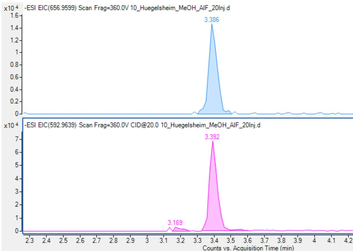
**Fig. S1.13** Top: EIC of 656.9599 (m/z of 12:2 FTUCA, 0 eV); bottom: EIC of 592.9639 (m/z of 12:2 FTUCA minus CO<sub>2</sub>HF, 20 eV)
