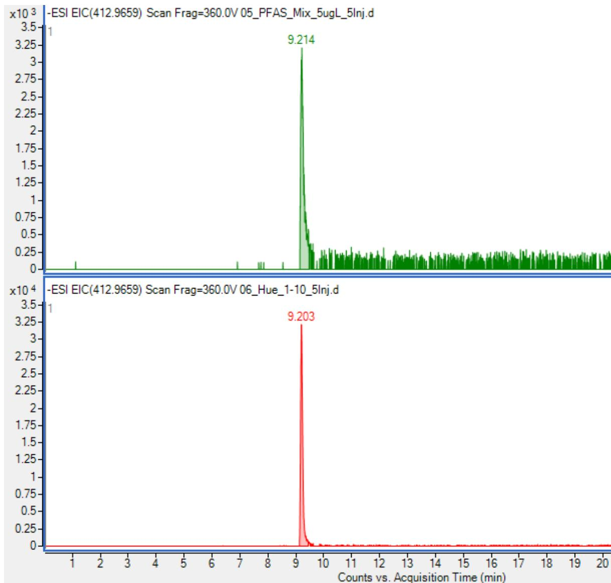
Fig. S1.1 Top: EIC of PFOA standard 5  $\mu\text{g/L}$ , bottom: 1/10 dilution of sample 1
