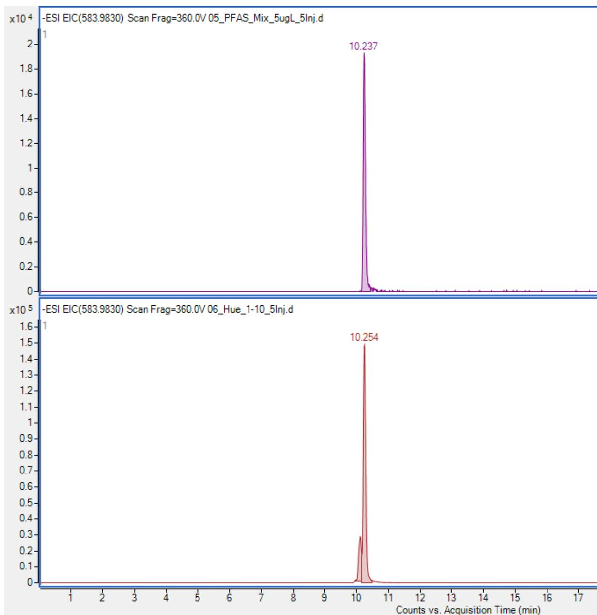
**Fig. S1.5** Top: EIC of EtFOSAA standard 5  $\mu\text{g/L}$ , bottom: 1/10 dilution of sample 1
