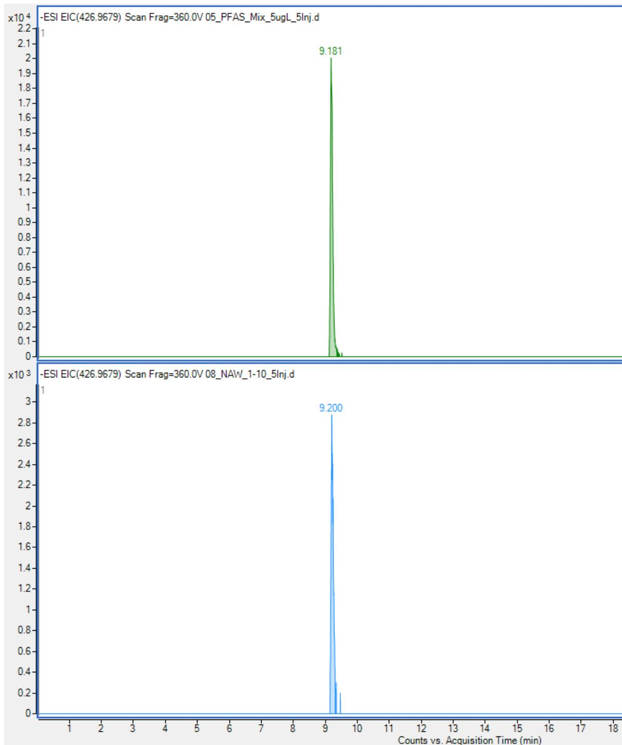
**Fig. S1.17** Top: EIC of 6:2 FTS standard 5 µg/L, bottom: 1/10 dilution of sample 2
