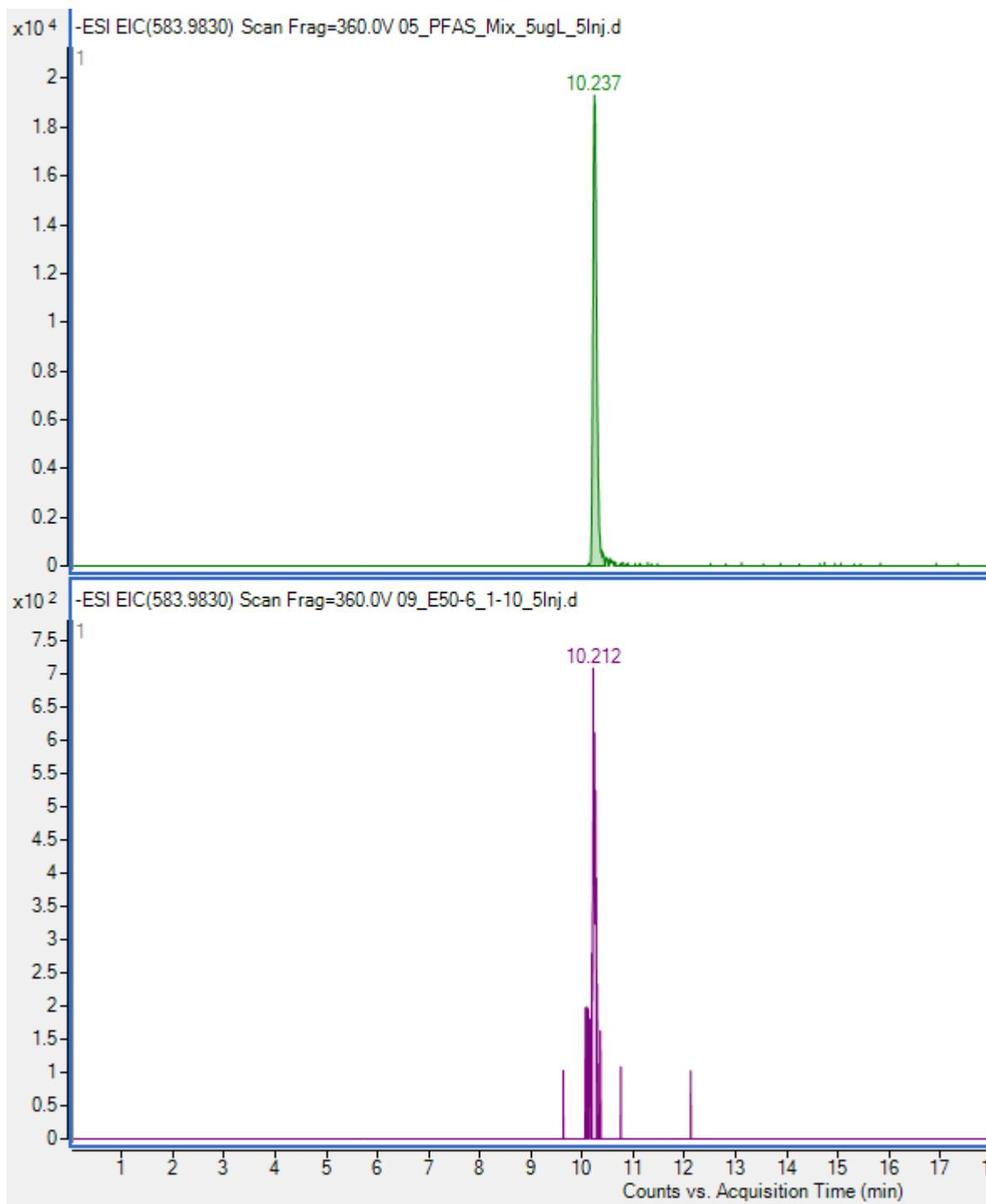
**Fig. S1.34** Top: EIC of EtFOSAA standard 5  $\mu\text{g/L}$ , bottom: 1/10 dilution of sample 4
