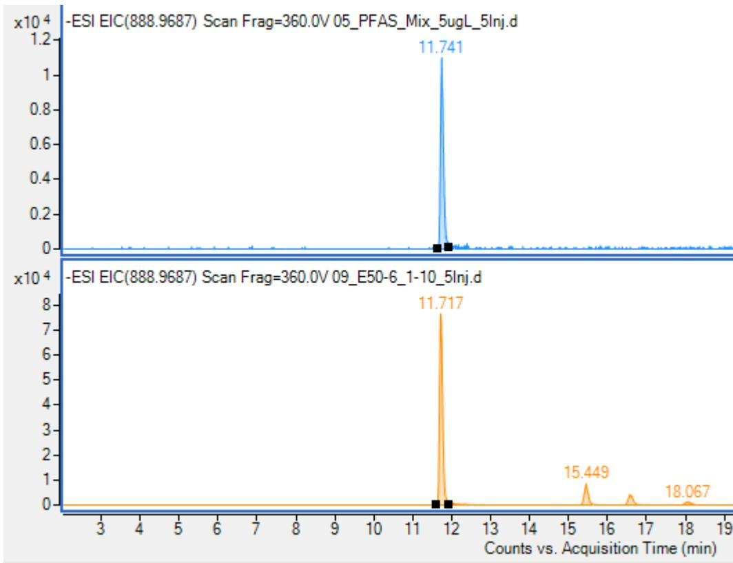
Fig. S1.51 Top: EIC of 6:2/8:2 diPAP standard 5  $\mu\text{g/L}$ , bottom: 1/10 dilution of sample 4
