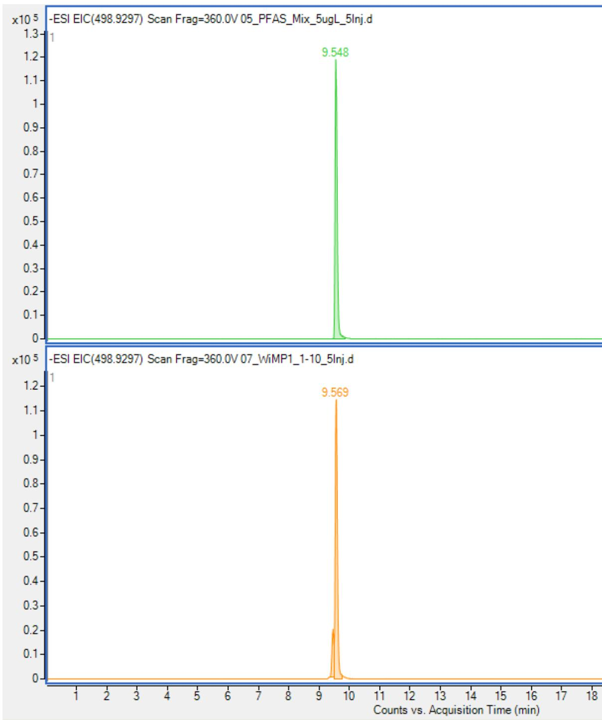
Fig. S1.26 Top: EIC of PFOS standard 5  $\mu\text{g/L}$ , bottom: 1/10 dilution of sample 3
