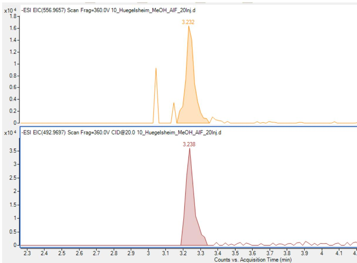
**Fig. S1.12** Top: EIC of 556.9657 (m/z of 10:2 FTUCA, 0 eV); bottom: EIC of 492.9697 (m/z of 10:2 FTUCA minus CO<sub>2</sub>HF, 20 eV)
