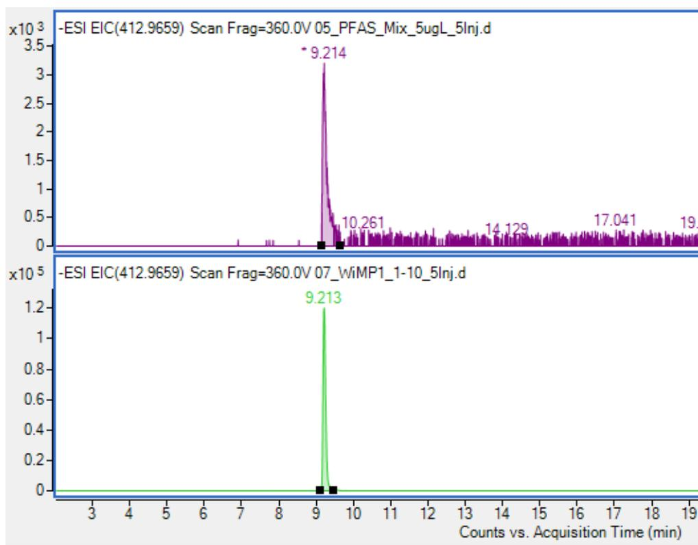
Fig. S1.48 EIC of PFOA standard 5  $\mu\text{g/L}$ , bottom: 1/10 dilution of sample 3
