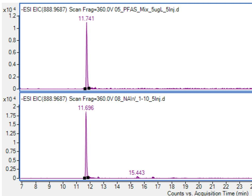
Fig. S1.47 Top: EIC of 6:2/8:2 diPAP standard 5 $\mu$ g/L, bottom: 1/10 dilution of sample 2
