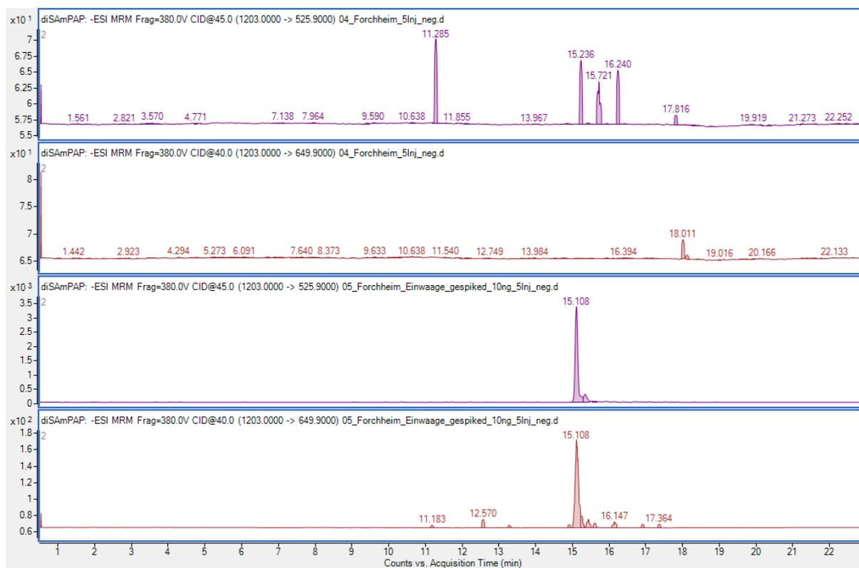
**Fig. S1.42** diSAmPAP (1203 -> 525.9, purple; 1203 -> 649.9, red). Top two chromatograms: uncontaminated soil sample, bottom 2 chromatograms: spiked uncontaminated soil sample
