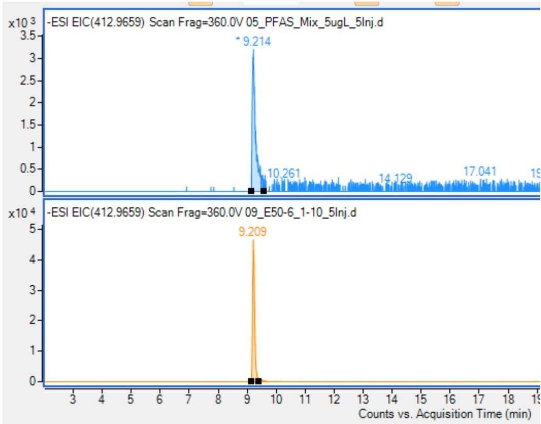
Fig. S1.50 Top: EIC of PFOA standard 5  $\mu\text{g/L}$ , bottom: 1/10 dilution of sample 4
