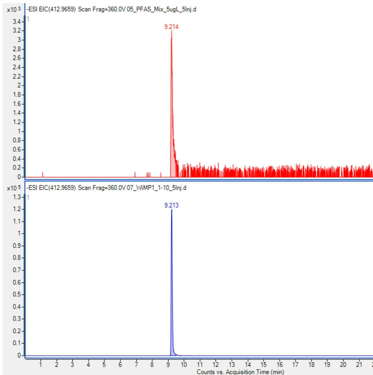
**Fig. S1.23** Top: EIC of PFOA standard 5  $\mu\text{g/L}$ , bottom: 1/10 dilution of sample 3
