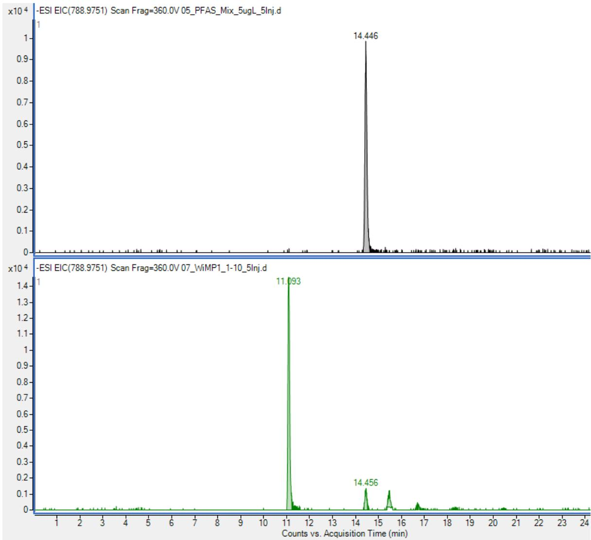
**Fig. S1.28** Top: EIC of 6:2 triPAP standard 5 µg/L, bottom: 1/10 dilution of sample 3
