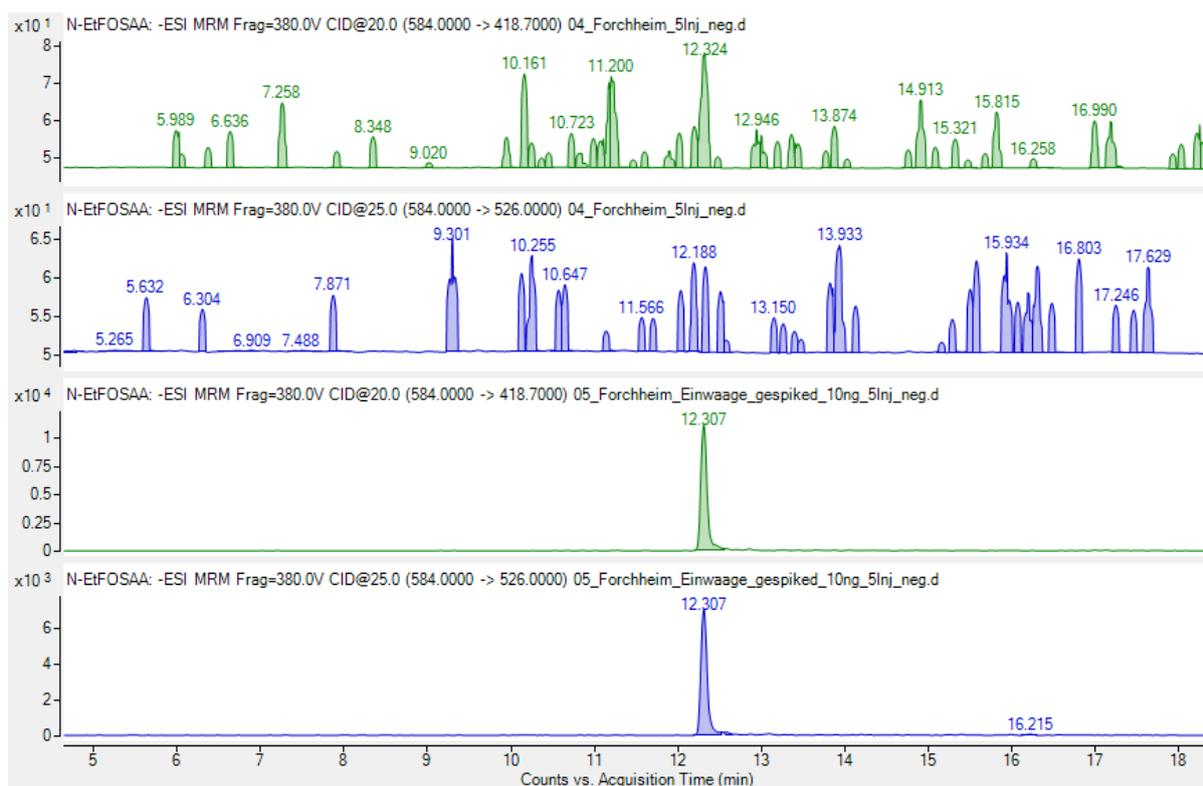
**Fig. S1.44** EtFOSAA (584 -> 418.7, green; 584 -> 526, blue). Top two chromatograms: uncontaminated soil sample, bottom 2 chromatograms: spiked uncontaminated soil sample
