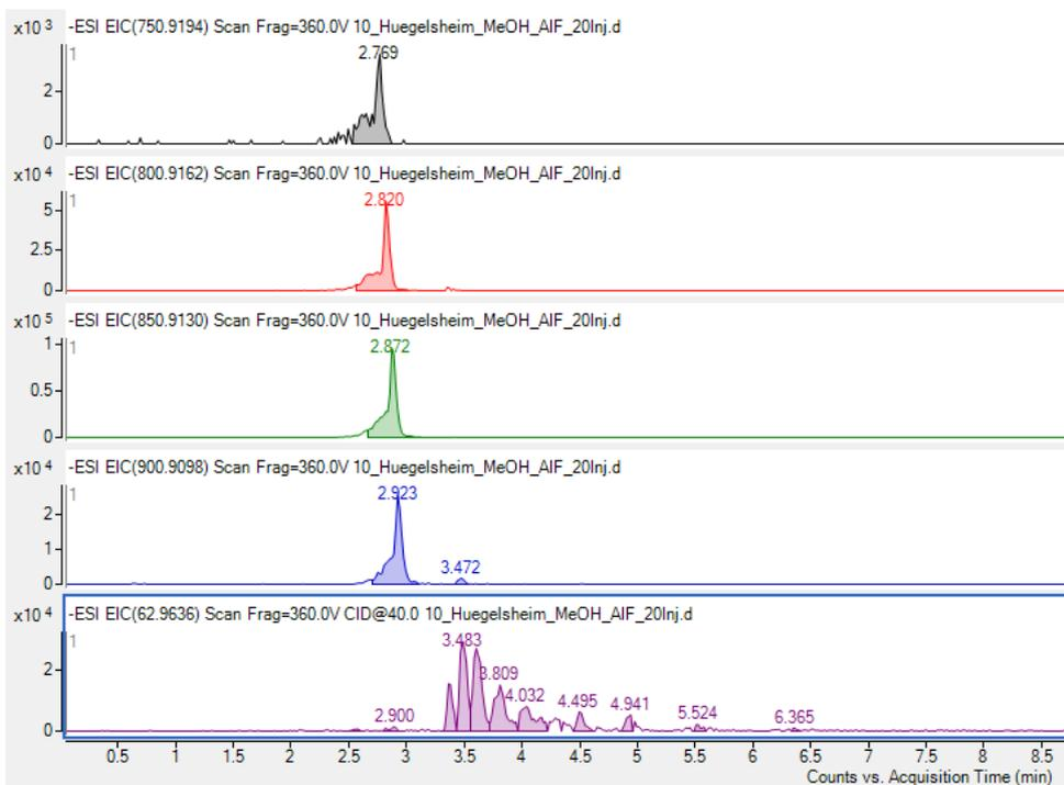
**Fig. S1.10** Chromatogram of PFPIA masses and the fragment  $m/z$  62.9638 @40 eV (AIF measurement). Chromatograms of  $m/z$  750.9194 (black), 800.9162 (red), 850.9130 (green), 900.9098 (blue) (these values fit the PFPIA substance class) and the fragment  $m/z$  62.9638 @40 eV (purple). No coelution can be observed
