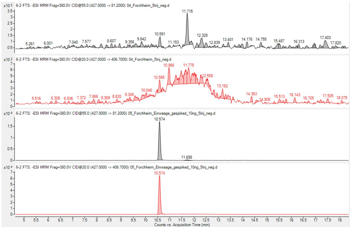
**Fig. S1.45** 6:2 FTS (427 -> 81.2, black; 427 -> 406.7, red). Top two chromatograms: uncontaminated soil sample, bottom 2 chromatograms: spiked uncontaminated soil sample
