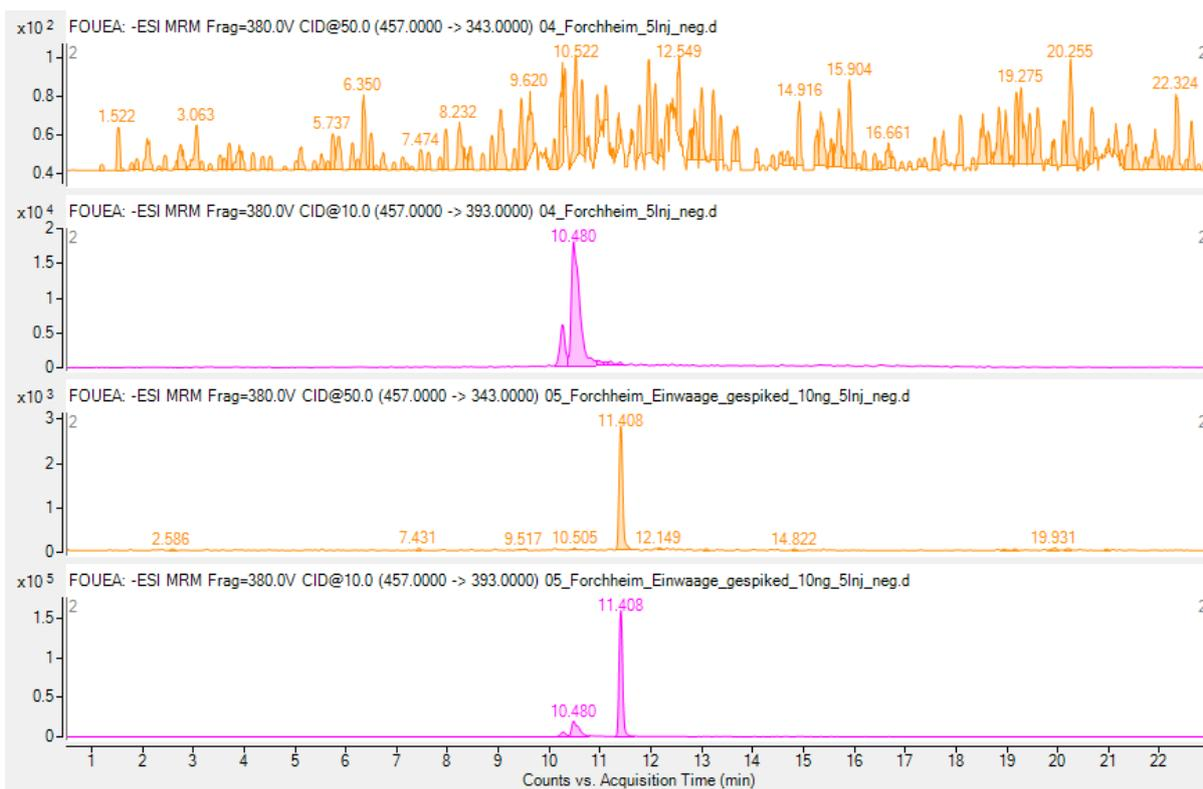
**Fig. S1.43** 8:2 PFCA (457 → 343, orange; 457 → 393, pink). Top two chromatograms: uncontaminated soil sample, bottom 2 chromatograms: spiked uncontaminated soil sample
