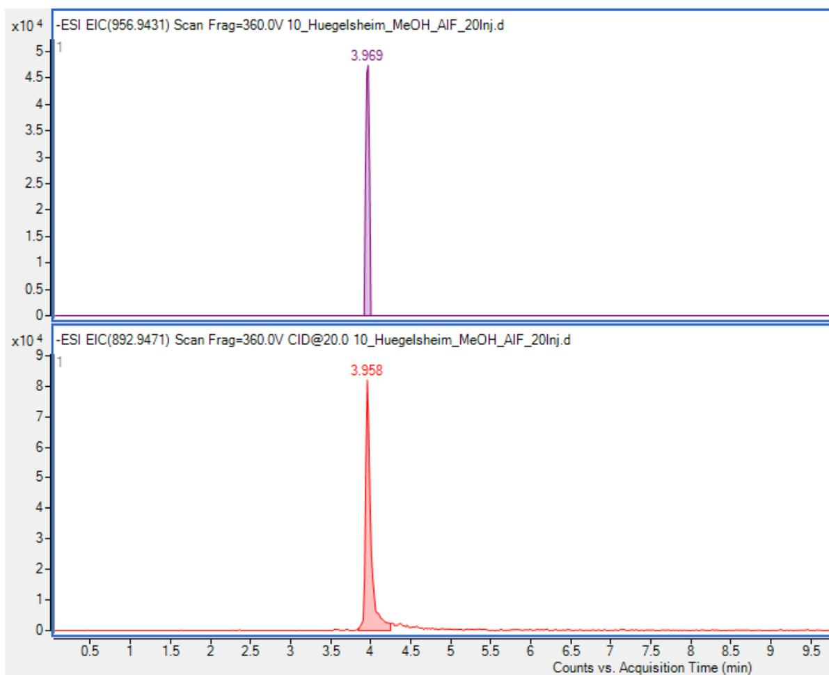
**Fig. S1.16** Top: EIC of 956.9431 (m/z of 18:2 FTUCA, 0eV); bottom: EIC of 892.9471 (m/z of 18:2 FTUCA minus CO<sub>2</sub>HF, 20 eV)
