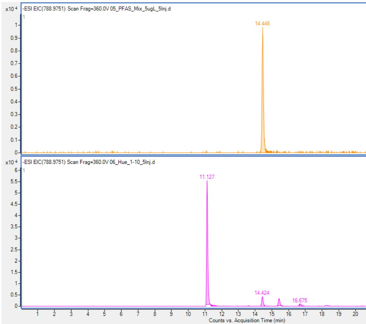
**Fig. S1.6** Top: 6:2 / 6:2 / 6:2 triPAP standard 5  $\mu\text{g/L}$ , bottom: 1/10 dilution of sample 1. The diPAP peak and further triPAP peaks in sample 1 are visible
