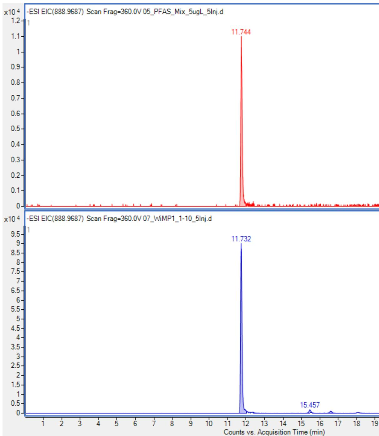
**Fig. S1.29** Top: EIC of 6:2 / 8:2 diPAP standard 5  $\mu\text{g/L}$ , bottom: 1/10 dilution of sample 3
