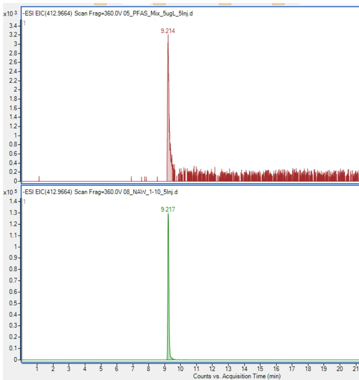
**Fig. S1.18** Top: EIC of PFOA standard 5  $\mu\text{g/L}$ , bottom: 1/10 dilution of sample 2
