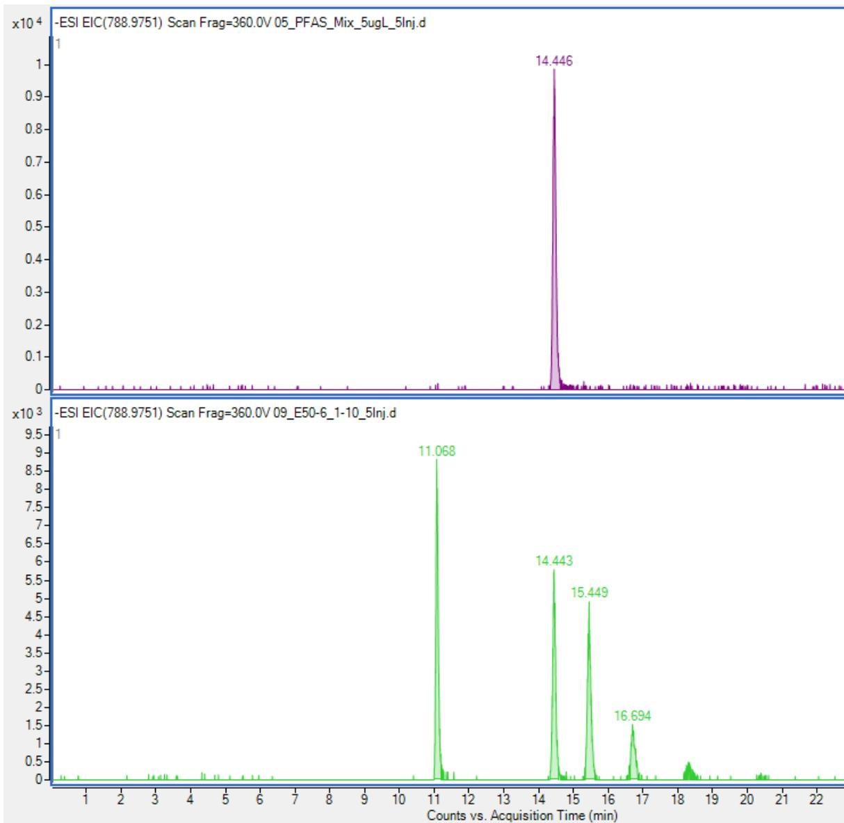
**Fig. S1.35** Top: EIC of 6:2 triPAP standard 5  $\mu\text{g/L}$ , bottom: 1/10 dilution of sample 4
