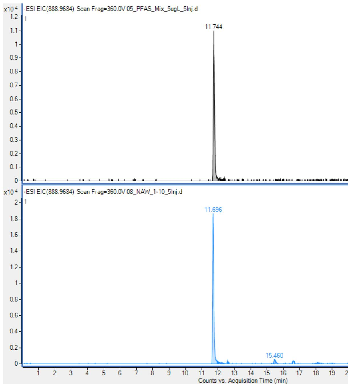
**Fig. S1.22** Top: EIC of 6:2 diPAP standard 5  $\mu\text{g/L}$ , bottom: 1/10 dilution of sample 2
