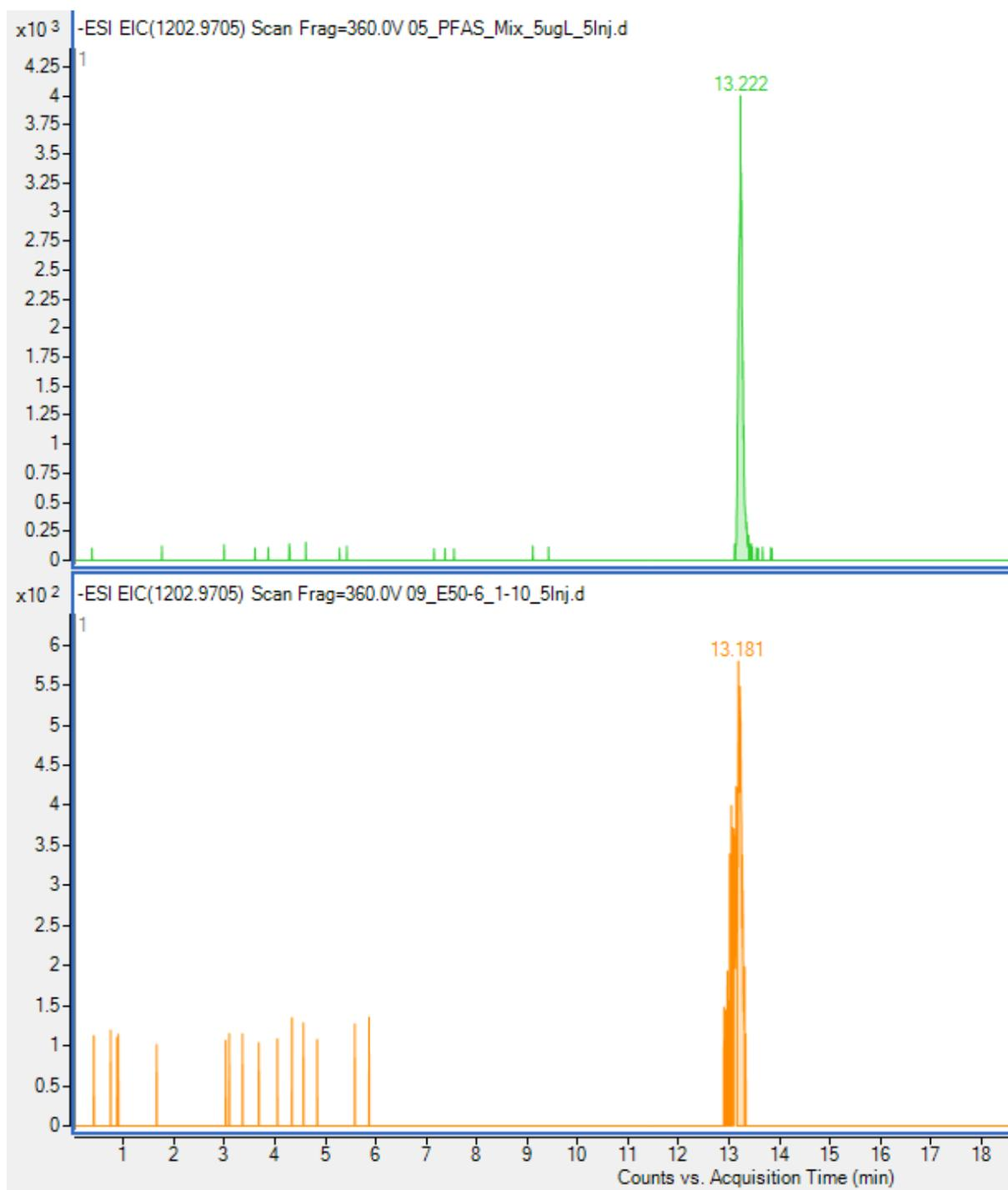
**Fig. S1.37** Top: EIC of diSAMPAP standard 5  $\mu\text{g/L}$ , bottom: 1/10 dilution of sample 4
