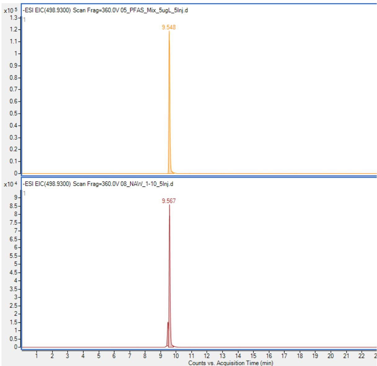
**Fig. S1.20** Top: EIC of PFOS standard 5  $\mu\text{g/L}$ , bottom: 1/10 dilution of sample 2
