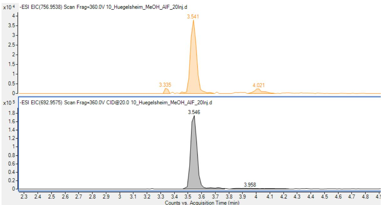
**Fig. S1.14** Top: EIC of 756.9538 (m/z of 14:2 FTUCA, 0eV); bottom: EIC of 692.9575 (m/z of 14:2 FTUCA minus CO<sub>2</sub>HF, 20 eV)
