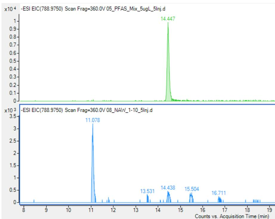
**Fig. S1.22b** Top: EIC of triPAP standard 5 $\mu$ g/L, bottom: 1/10 dilution of sample 2
