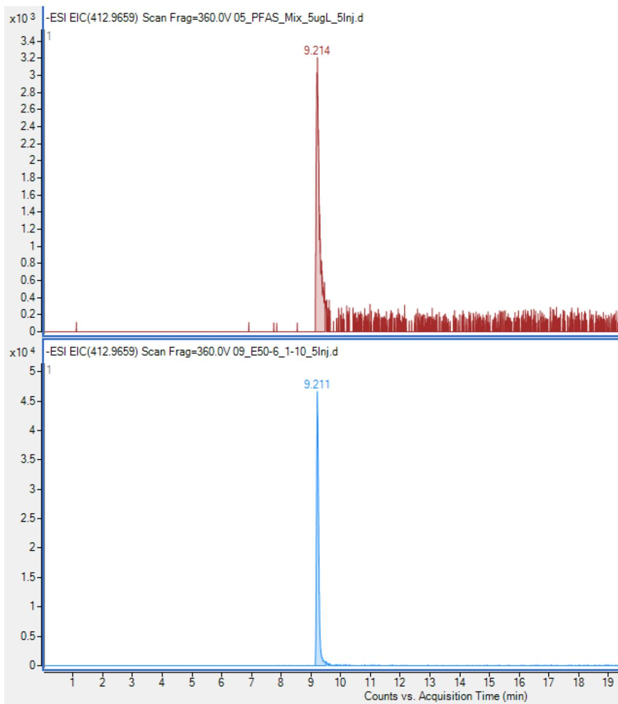
**Fig. S1.31** Top: EIC of PFOA standard 5  $\mu\text{g/L}$ , bottom: 1/10 dilution of sample 4
