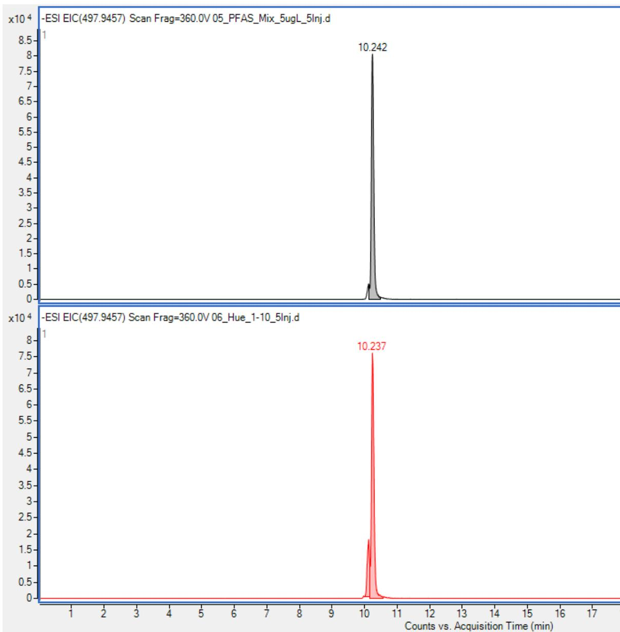
**Fig. S1.3** Top: EIC of FOSA standard 5  $\mu\text{g/L}$ , bottom: 1/10 dilution of sample 1
