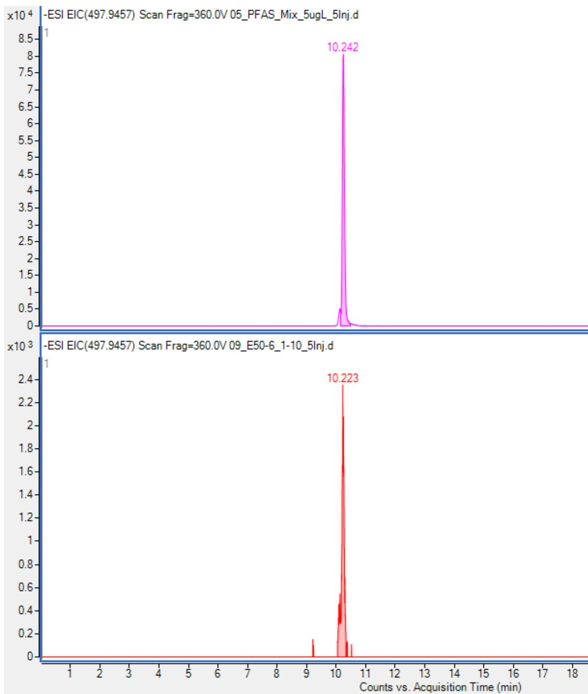
**Fig. S1.32** Top: EIC of FOSA standard 5  $\mu\text{g/L}$ , bottom: 1/10 dilution of sample 4
