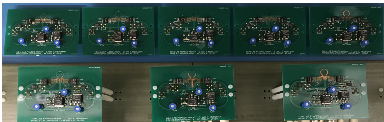
(a) Photograph of 8 phase-tunable oscillators built and measured.
