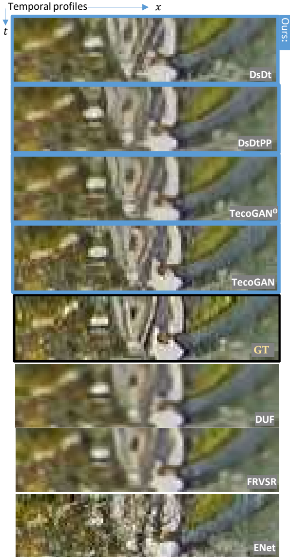
Figure 7. Calendar scene comparisons as temporal profiles (time shown along y axis). Our TecoGAN models lead to natural temporal progressions, and our final model closely matches the desired ground truth behavior over time.
