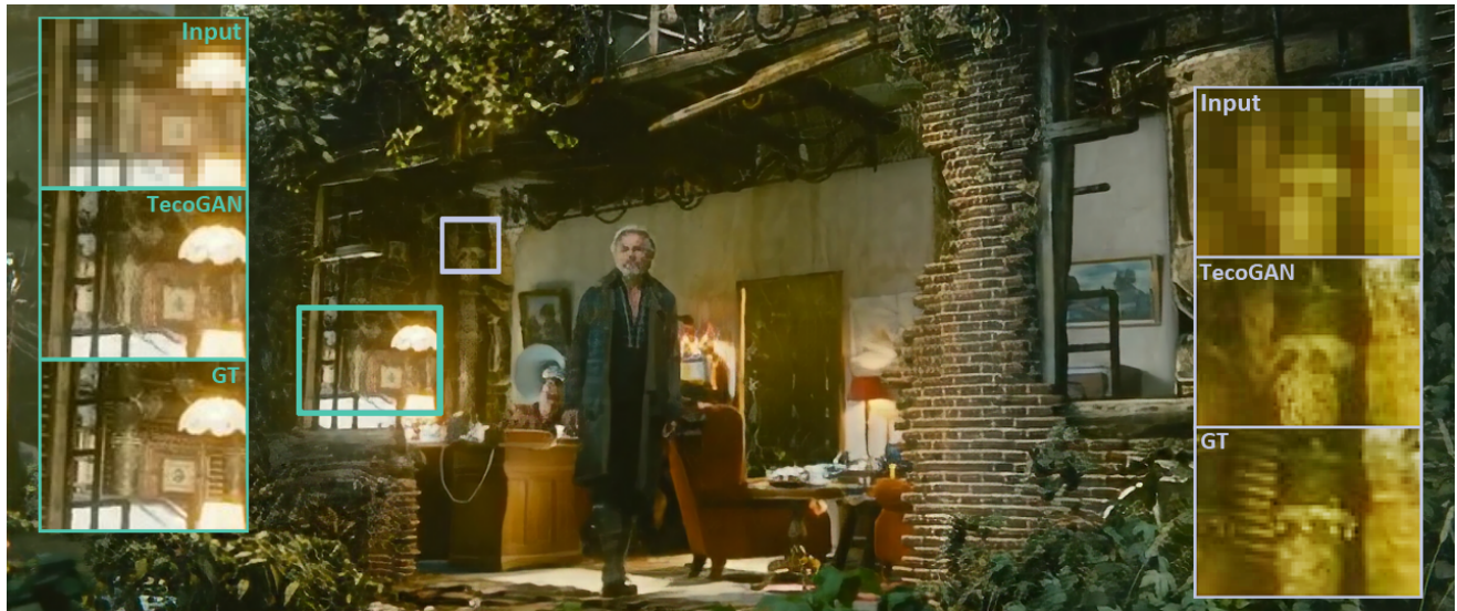
Figure 1. Our temporally coherent video super-resolution GAN can generate sharp, coherent and realistic results. Here we show the low-resolution inputs, our results and the high-resolution ground truth images for the Tears of Steel [5] room scene, from top to bottom.
