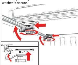
Unfold the cover (C) towards the tailgate. Then confirm each panel is centered side to side and front to back on the truck bed. If adjustments are needed, loosen the cover retainer clamps (F) and shift the cover (C) until positioned correctly. Retighten the cover retainer clamps once the desired fitment is reached. If adjustments to the slam latch are needed, see the directions on the next page.
