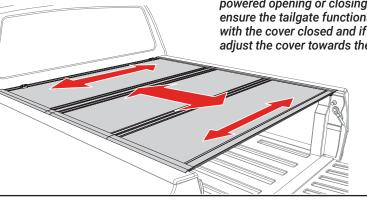
The rear edge of the cover (C) and tailgate seal should rest on top of the tailgate. You are ready to drive with your cover in the closed position.
