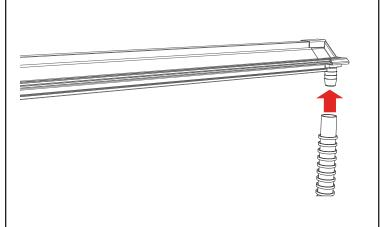
Place the passenger side rail (A) on the truck rail. Position the side rail flush with the top edge of your truck bed rail. The end of the side rail with the drain tube will go towards the cab of the truck. Repeat on the opposite side with the driver's side rail (B).
