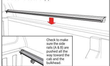
Attach three clamps (G) to the driver side rail (B) to the truck bed. Place the front clamp 6-8 inches from the bulkhead. Place the rear clamp as close to the tailgate as possible. Center the middle clamp accordingly. Clamps should be evenly spaced along the full length of the rail. Loosely tighten with a 1/2" wrench to make sure the clamps engage with the side rail. Repeat on the passenger side rail (A).
