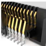
Edge Rate® contacts optimized for superior signal integrity performance
