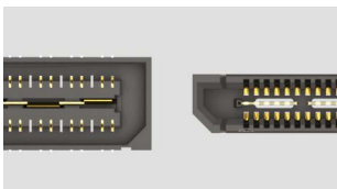
Slim 4.60 mm body width saves board space
