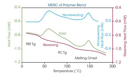
The plot shows MDSC results for a thermoplastic alloy blend of polycarbonate (PC) and polybutylene terephthalate (PBT). This material exhibits a variety of overlapping transitions, and interpretation of the Total Heat Flow is complicated. MDSC effectively separates the crystallization of the PBT component into the Non-Reversing Heat Flow, thereby allowing for accurate determination of the glass transition temperatures of each polymer in the Reversing Heat Flow.
