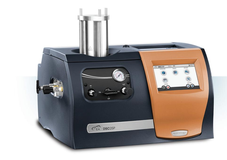
The DSC 25P is a dedicated Pressure DSC that provides heat flow measurements on pressure sensitive materials. The Discovery DSC 25P is used to study thermal transitions, chemical reactions, oxidative stability and decomposition under vacuum, atmospheric pressure and elevated pressures.
