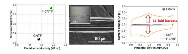
A comparison of the mechanical and electrical conductivity property enhancement of functionalized carbon nanotube fiber compared to raw fiber, showing a 33-fold increase in electrochemical activity despite a clean surface with no active material. Credit: Korea Institute of Science and Technology
