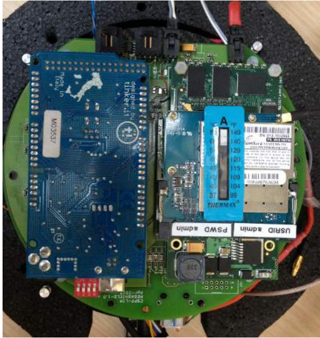
Figure 9: The Arduino board running the position controller and the on-board radiomodem attached on their carrier board.
