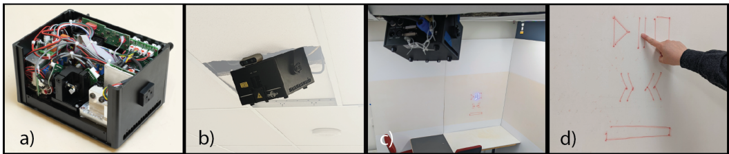
Fig. 5. Panel a) A custom modified 405 nm laser vector projector, which provides wide array coverage from long distances. Panel b) A view of the laser projector and depth camera mounted to the ceiling. Panel c) The ceiling mounted laser projector projecting an image, a music menu, onto the wall. Panel d) A closeup of the music menu projected onto the wall.
