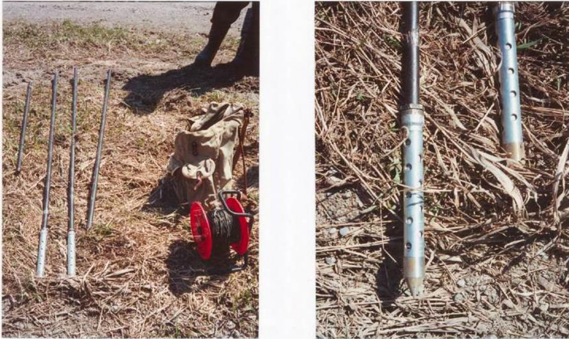
Figure 2: Typical construction of mini-piezometers (left) and mini-piezometer tips (right).
