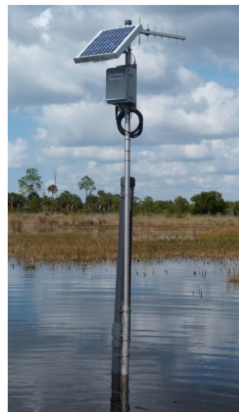
Figure 10.1: An in-water turbidity monitoring station.
