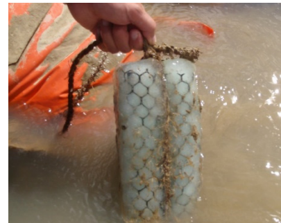
Figure B2-25: Polymer flocculant in gel-block form
