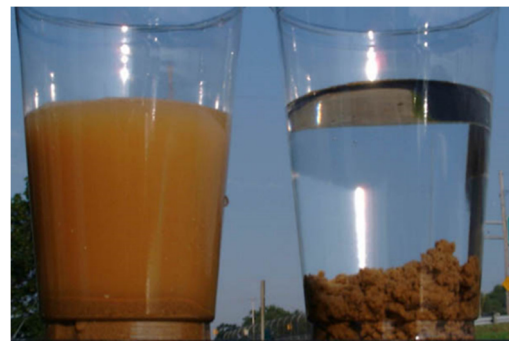
Figure B2-24: Turbidity reduction in water sample following treatment with a flocculant. Before on the left and after on the right.
