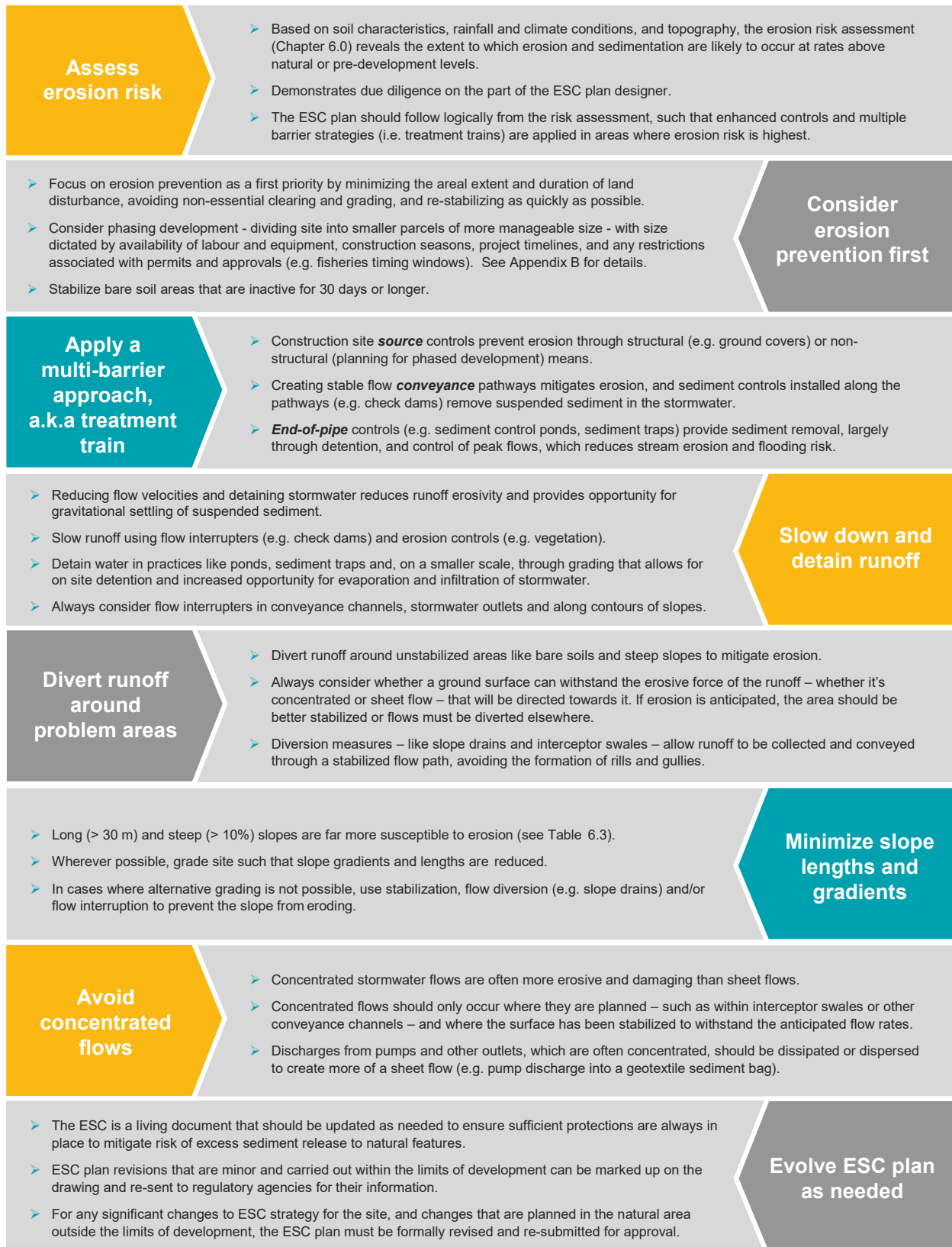
Figure 7.1: Principles of ESC planning
