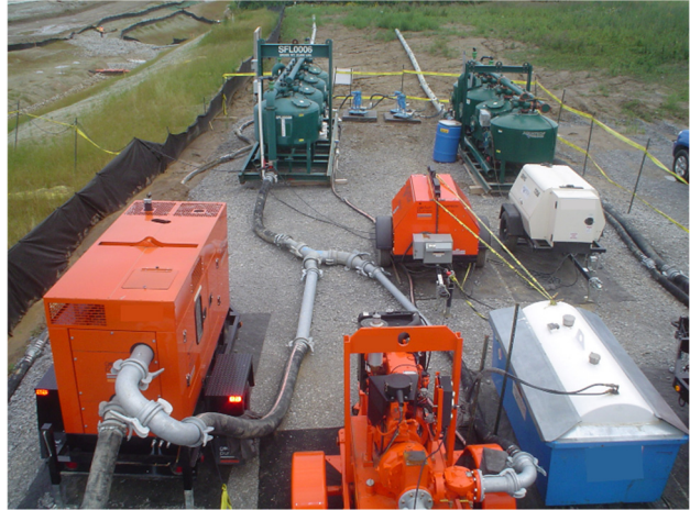
Figure 7.13: Active treatment system
