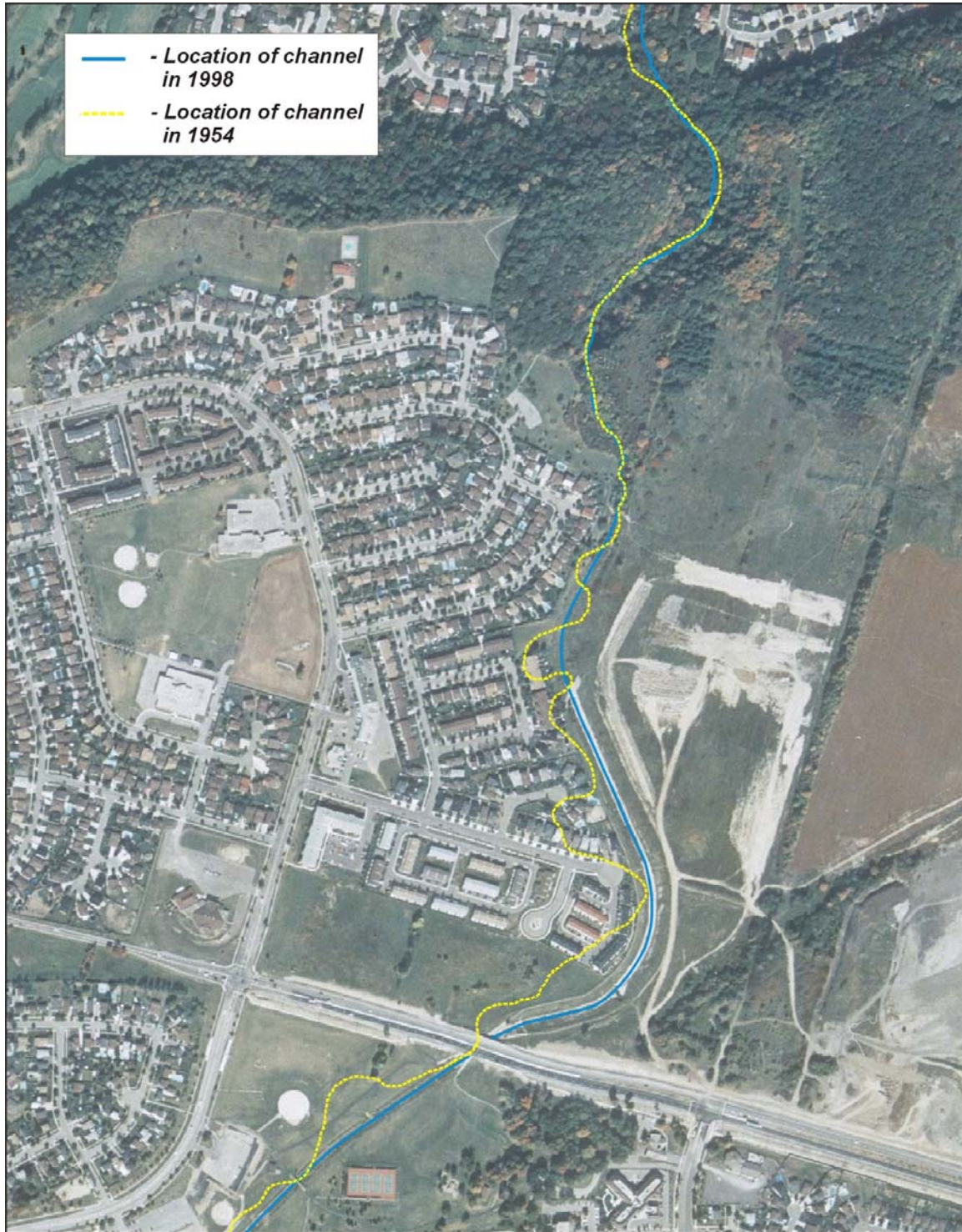
Figure 5.2: When an altered reach no longer occupies its potential meander belt, a reference to historic air photos or mapping often shows the natural configuration.
