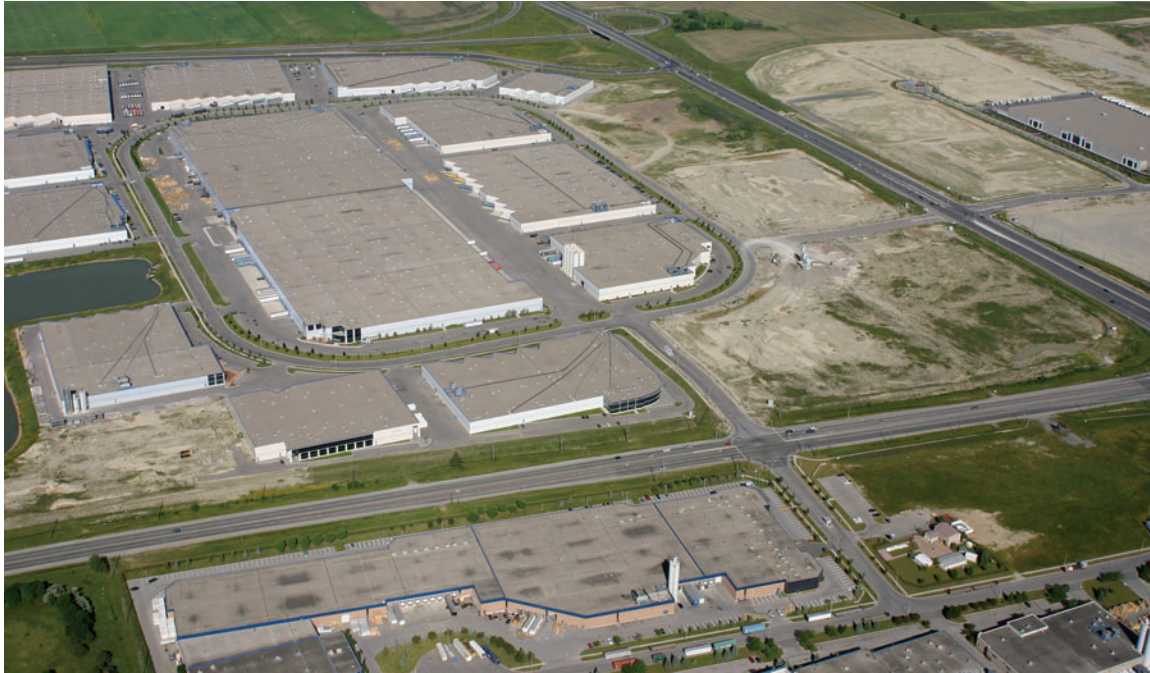
Industrial and commercial developments typically create extensive areas of hard (impervious) surfaces that greatly increase stormwater run-off. Photography by Lou Wise
