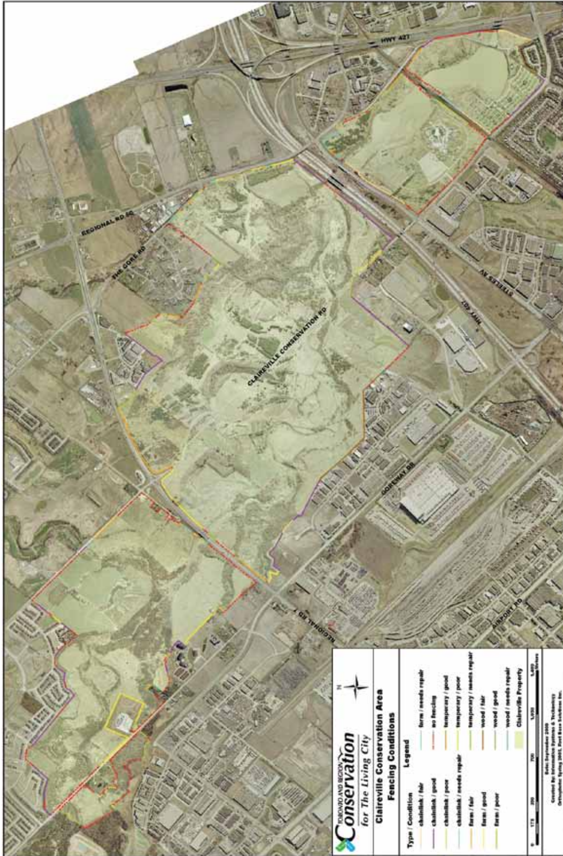
Map G.4: Existing fencing types and conditions, Site Securement and Protection Plan, Claireville Conservation Area
