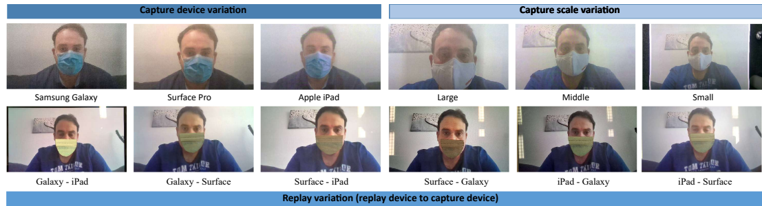
Figure 4.2.: Different capture variations in the CRMA database. The top left shows the videos captured by different devices. The top right shows the different capture scales. The bottom shows the six cross-device types of replay attack settings.
